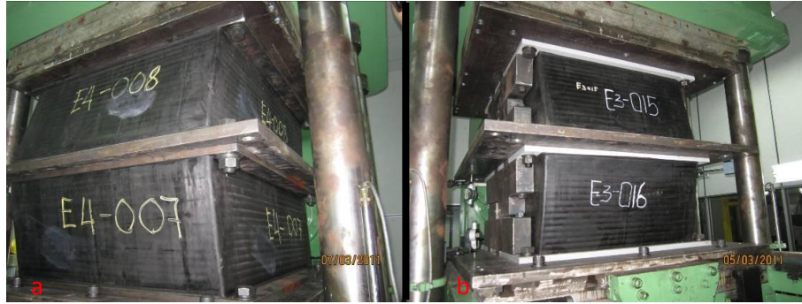
Figure 6. Tests in double shear configuration: a) Left: bearings without preset plates, b) Right: bearings with preset plates installed after test.
