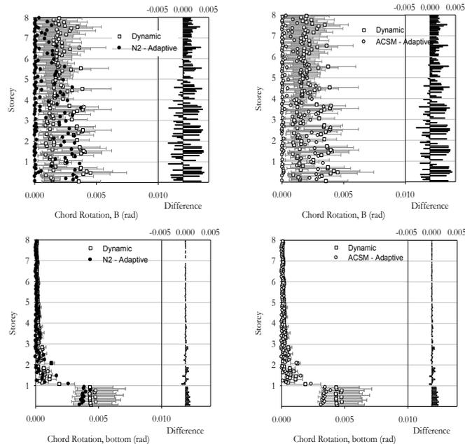
**Figure 3.6.** Beams' (top) and columns' (bottom) chord rotations for the 8-storey building analysed under static (N2 method, ACSM) and dynamic analyses, in Y directions.
