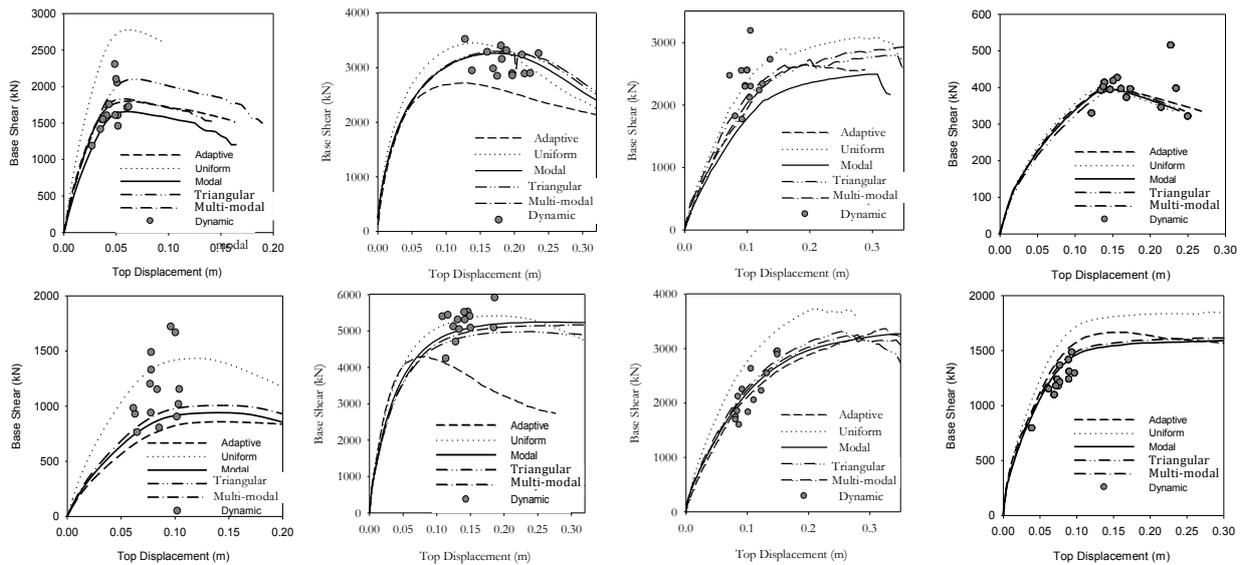
**Figure 3.1.** Capacity curves and dynamic performance for 2-, 4-, 5- and 8-storey building (left to right), assuming the most realistic simulation, in X (top) and Y (bottom) directions.
