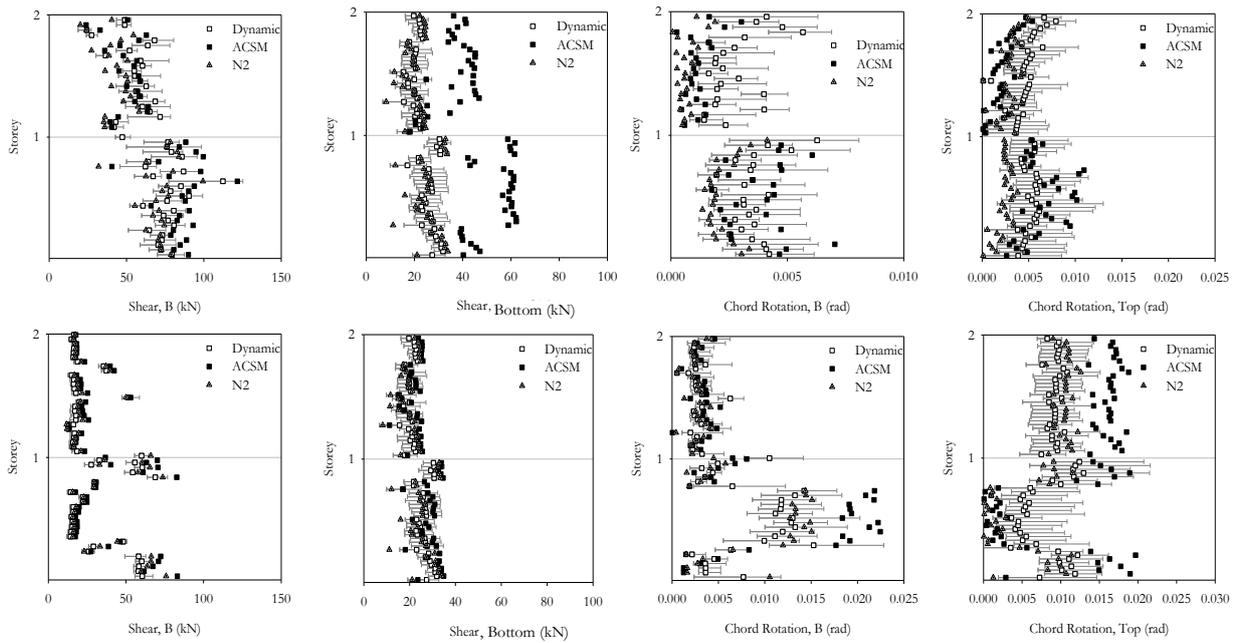
**Figure 3.3.** Beams and columns shear forces and chord rotations measured for the 2-storey building, analysed under static (ACSM and N2-modal distribution) and dynamic analyses in X (top) and Y (bottom) directions.
