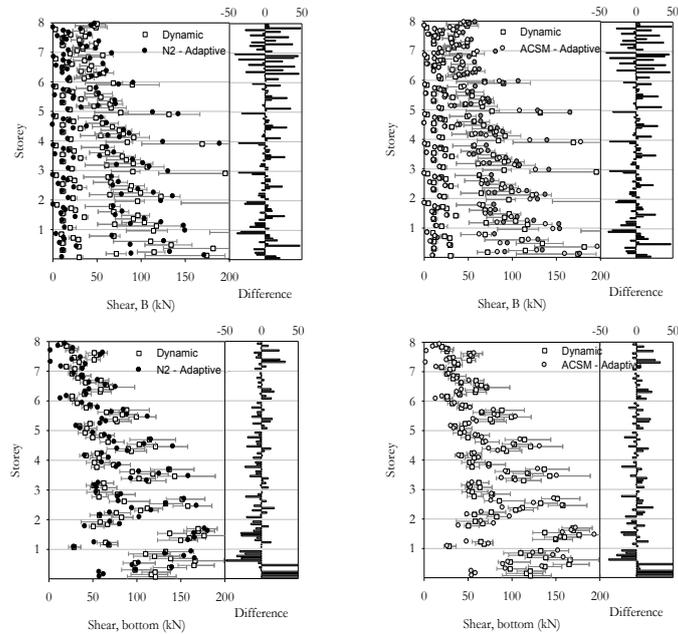
**Figure 3.5.** Beams' (top) and columns' (bottom) shear for the 8-storey building analysed under static (N2 method, ACSM) and dynamic analyses, in X directions.
