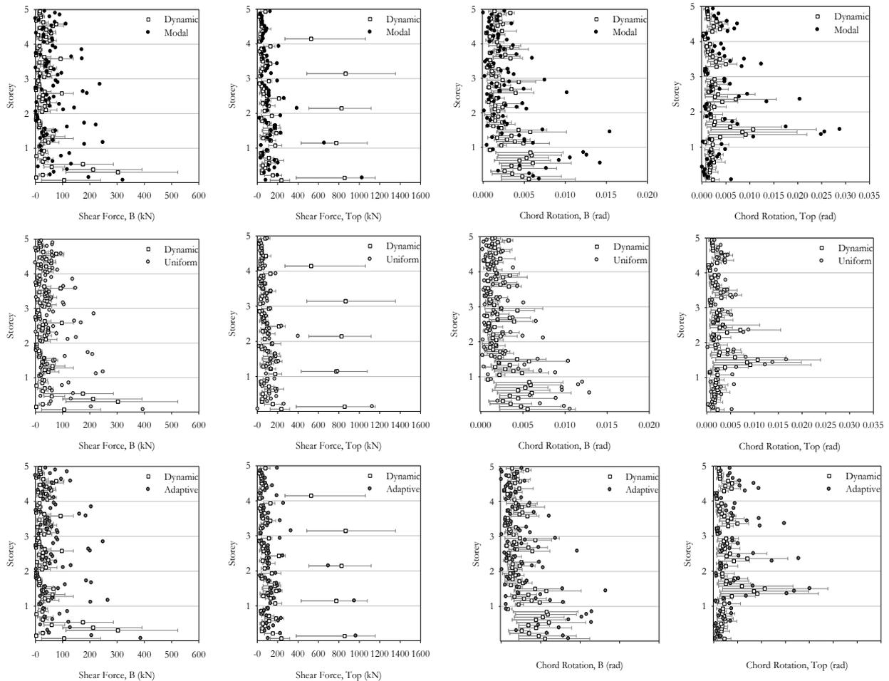
**Figure 3.2.** Beams' (1<sup>st</sup> and 3<sup>rd</sup> column) and columns' (2<sup>nd</sup> and 4<sup>th</sup> column) shear forces and chord rotations for the 5-storey building analysed under static (N2 method with different load distributions) and dynamic analyses, in X directions.
