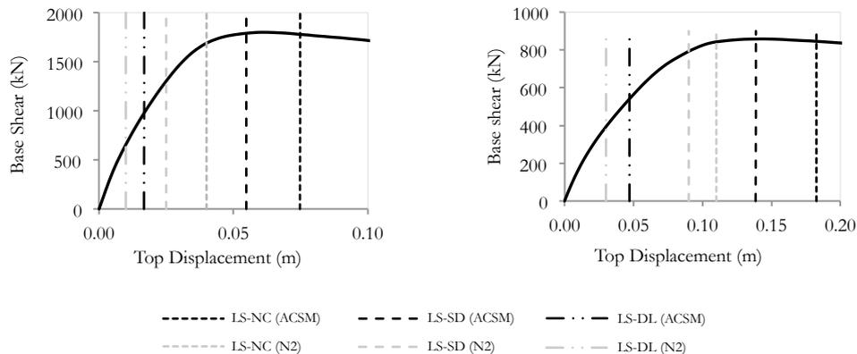
**Figure 3.4.** Performance points resulting from the application of the N2 method and ACSM for the 2-storey building in X (left) and Y (right) directions.
