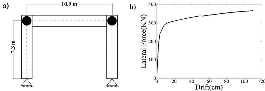
**Figure 2.3** (a) Schematic dimensions for the frame (b) pushover analysis results.
