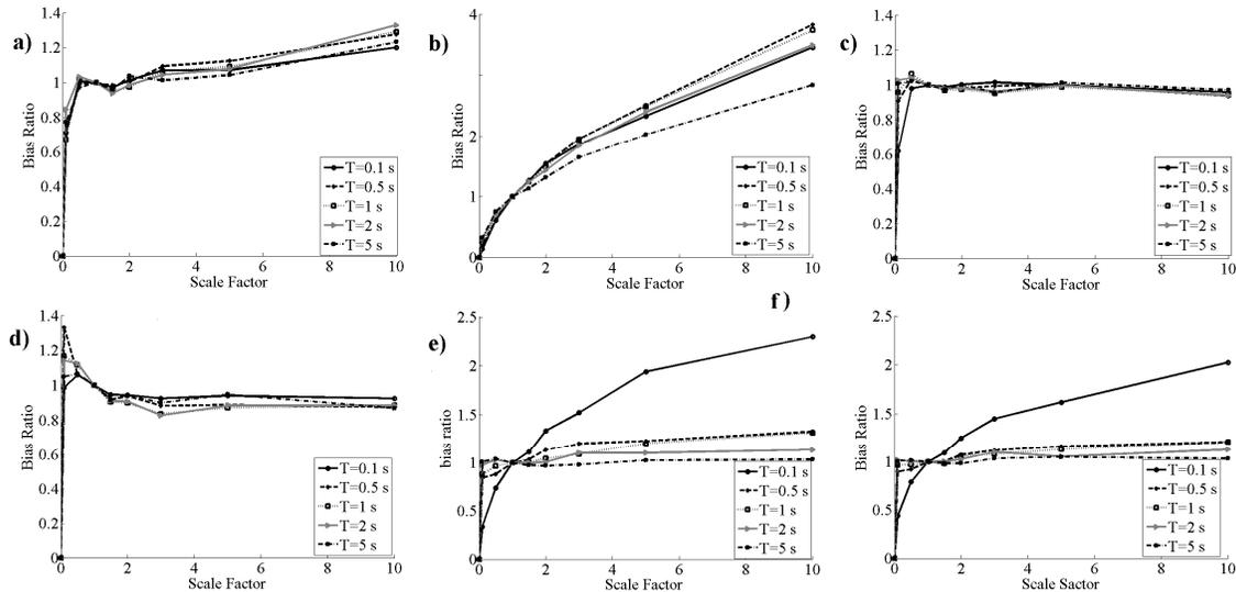
**Figure 3.2** (a) to (e); bias values for synthetic ground motions and elasto-plastic system for binning based on PGA, IA, PGV, CAV and SD respectively. (f); for binning based on SD and bilinear system with hardening ratio equal to 20%.
