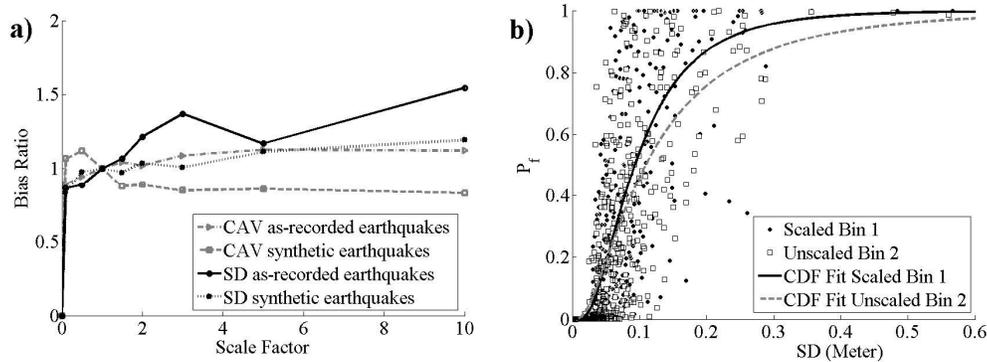
**Figure 3.3** (a) bias values of frame for binning based on SD and CAV (b) Fragility curves for the frame associated to scaled and unscaled bins for bias value equal to 1.37.
