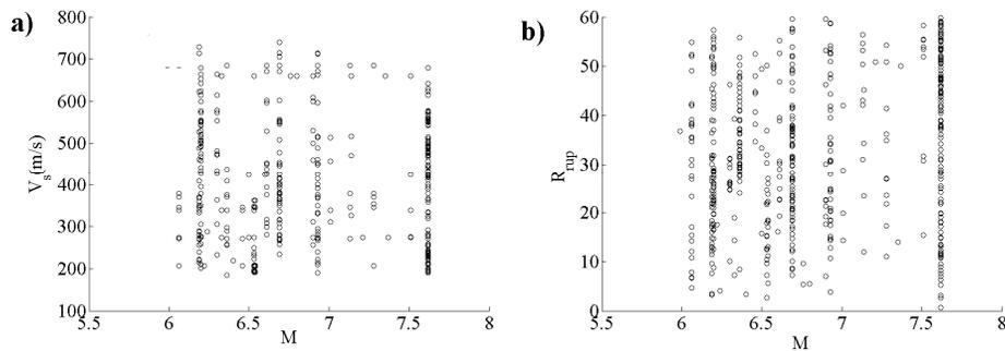
**Figure 2.1** (a) Distribution of moment  $M$  versus  $R_{rup}$  and (b) Distribution of moment  $M$  versus  $V_{s30}$  for selected records
