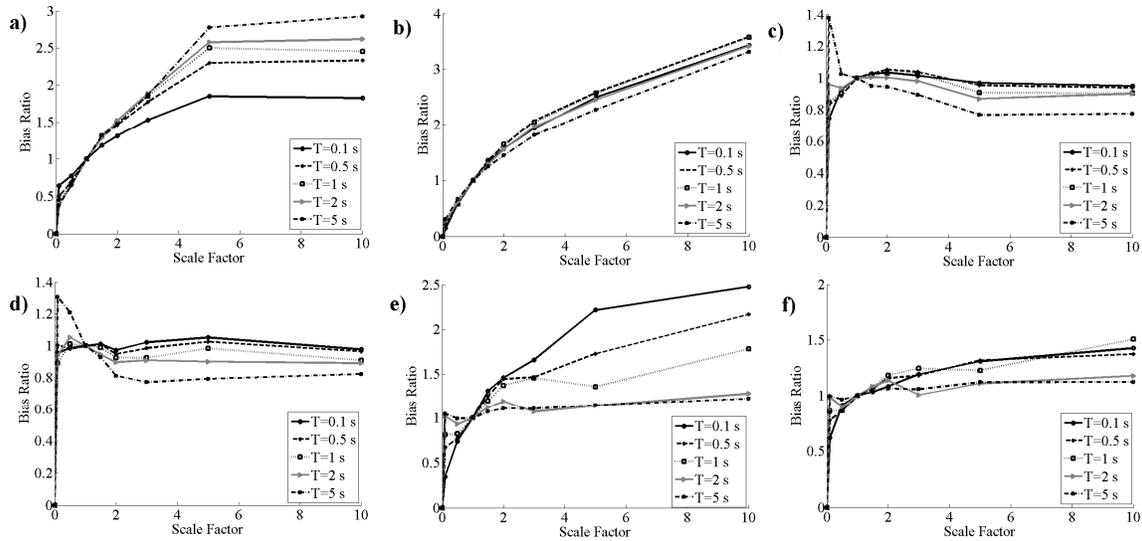
**Figure 3.1** (a) to (e); bias values for as-recorded ground motions and elasto-plastic system based on PGA, IA, PGV, CAV and SD respectively. (f); for binning based on SD and bilinear system with hardening ratio equal to 20%.
