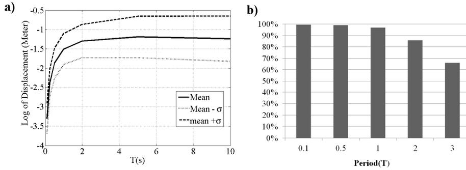
**Figure 2.2** (a) Mean and mean  $\pm\sigma$  response spectrum. (b) Percentage of yielding observed for SDOF system with  $F_y=0.2$  N.
