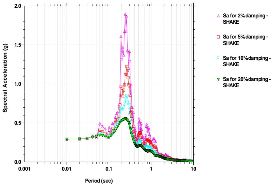
Figure 3.3. Response Spectra at 2, 5, 10 & 20% damping
