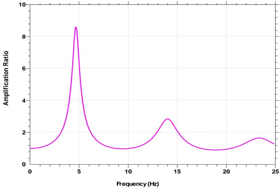
**Figure 3.4.** Amplification Spectrum
