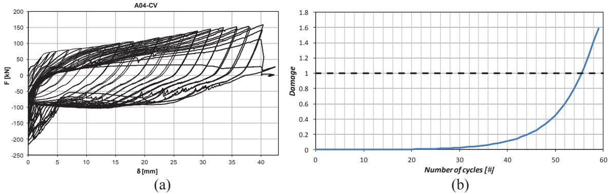
**Figure 7.** Hysteresis loops of specimen under variable cyclic test and cumulative damage
