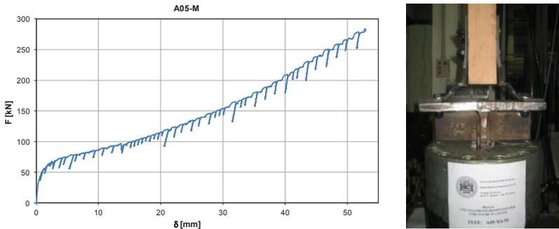
Figure 3. Monotonic curve and test setup for tension testing of L-stubs connections
