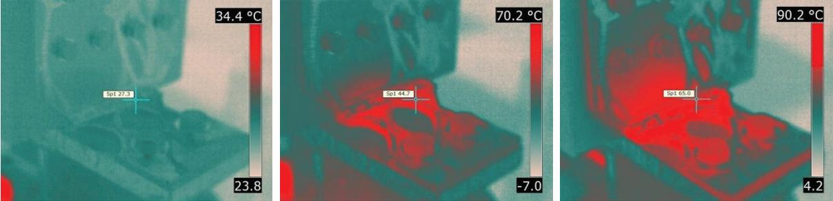
Figure 5. IR camera pictures of the L-stub up to the sixth cycle at 25 mm of amplitude
