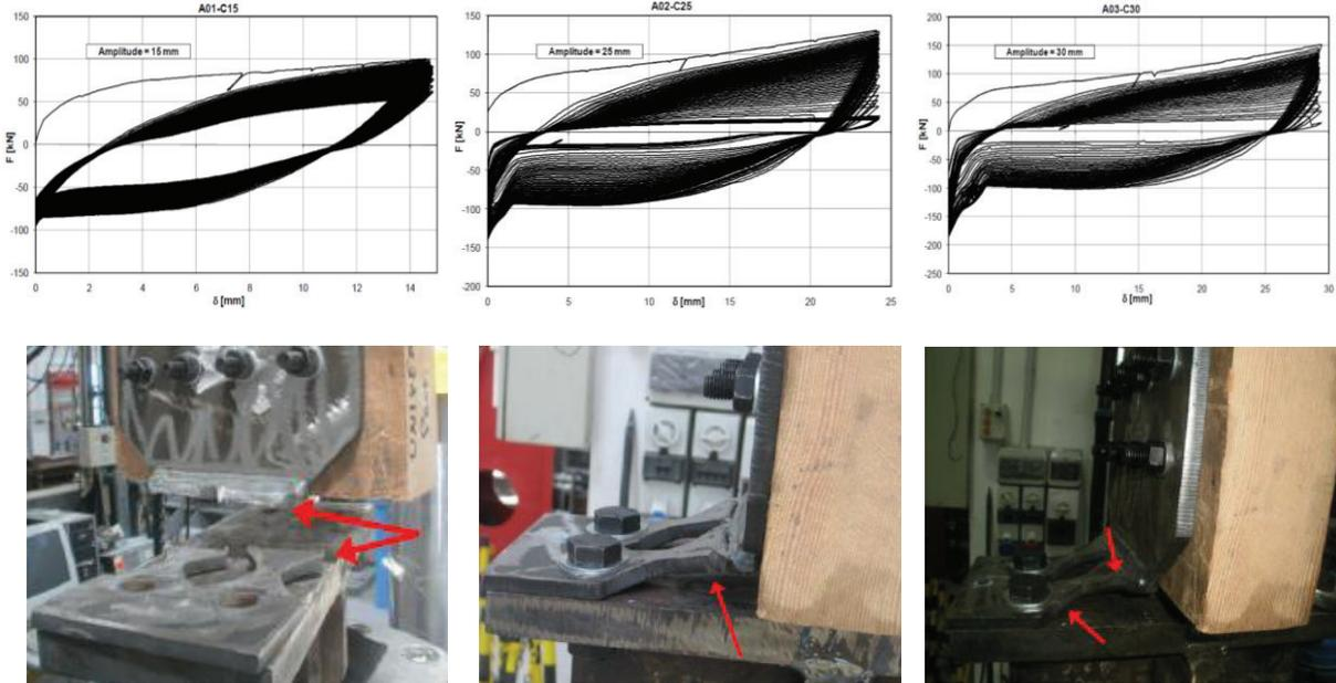
Figure 4. Hysteresis loops and failure mode of a couple of XL-stubs in constant amplitude cyclic tests
