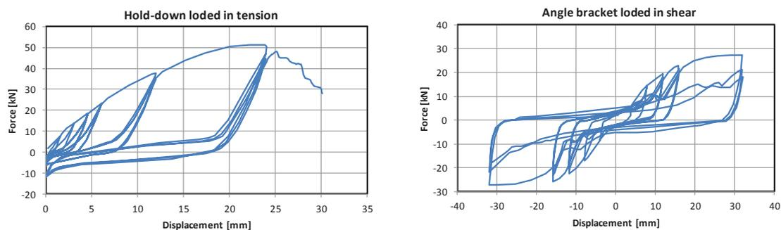
**Figure 2.** Hysteresis loops of a hold-down loaded in tension and of an angle bracket loaded in shear
