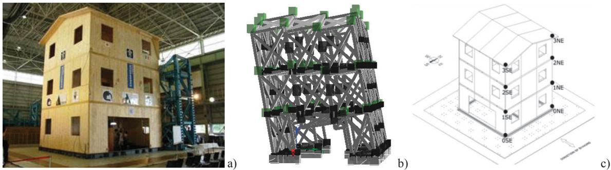
**Figure 8.** a) Real building; b) deformed configuration of the numerical model; c) points of control of displacements
