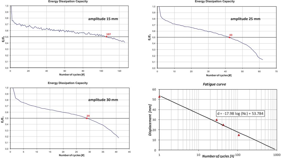
Figure 6. Conventional collapse of specimens under constant amplitude cyclic tests and fatigue curve
