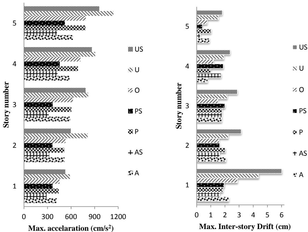
**Figure 5.1.** The maximum absolute acceleration and inter-story drift in the five-story structure
