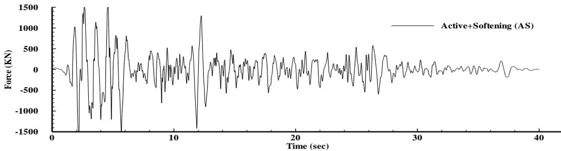
**Figure 5.2.** Device force in the AS case (first floor)
