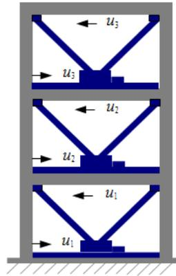
**Figure 3.1.** Distribution of the actuators in the three-story structure
