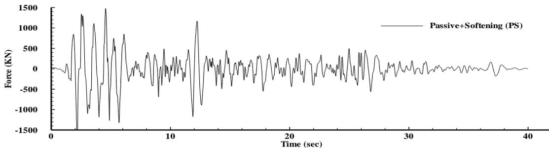
**Figure 5.3.** Device force in the PS case (first floor)
