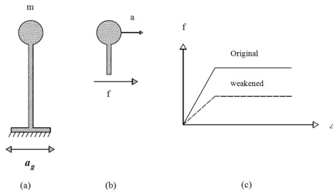
**Figure 2.1.** Weakening and softening in a single-degree-of-freedom system.
