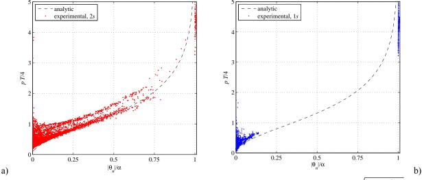
Figure 5. Non-dimensional period of the wall, *T*, multiplied by the frequency parameter  $p = \sqrt{m g R/I_o}$ . Comparison between experimental data and analytical formulation (Housner 1963).
