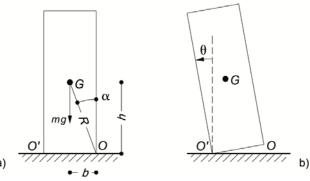
Figure 1. Parapet wall: geometrical parameters and displaced configuration.
