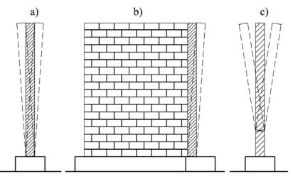
Figure 3. a) Two-sided rocking, b) one-sided rocking, c) wall fractured above the base in order to get a different height-to-thickness ratio
