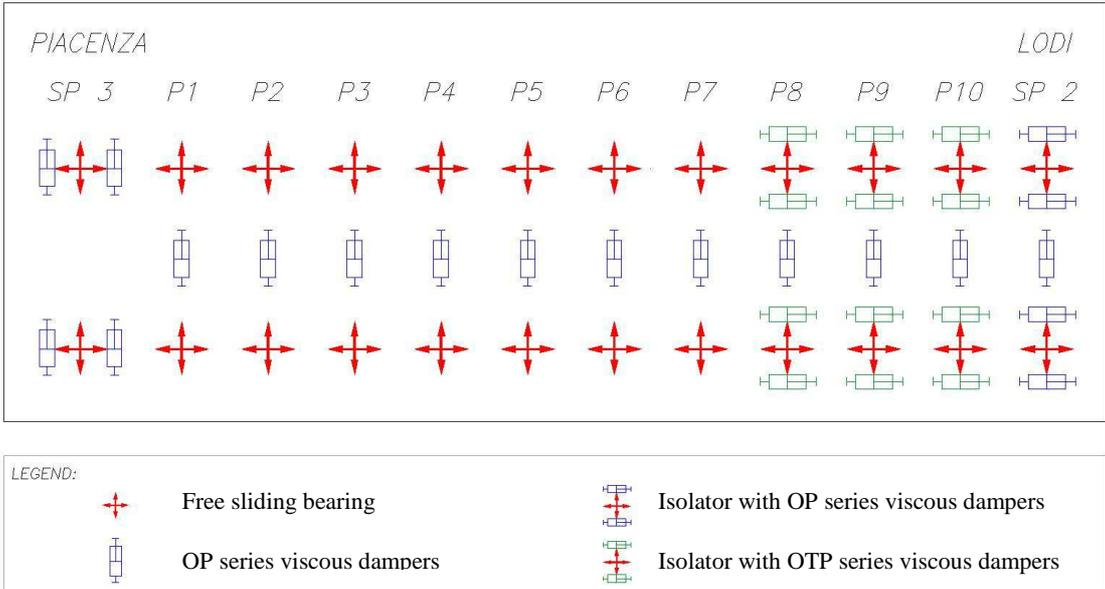
**Figure 3.** Seismic isolation system layout of the main bridge over Po river in Piacenza.
