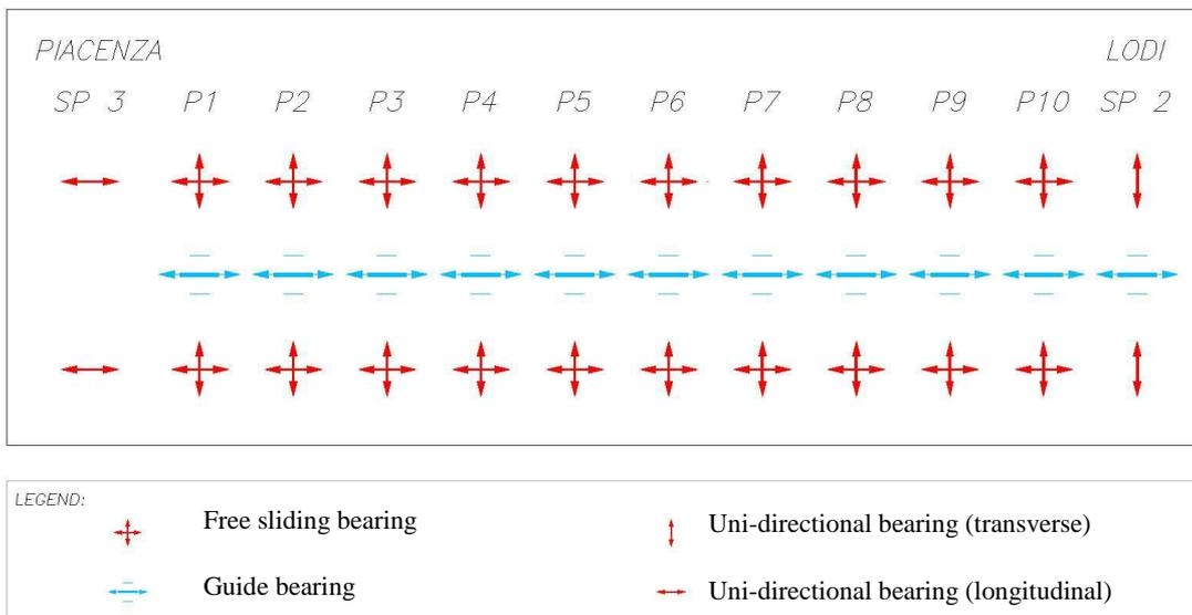
**Figure 6.** Bearing layout of the main bridge over Po river in Piacenza under service movements.
