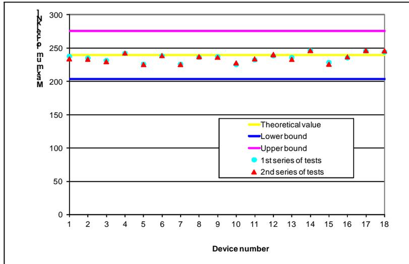
**Figure 8.** Maximum force (average of the 5 cycles of each series of tests) for the 18 viscous dampers subjected to FPCT.
