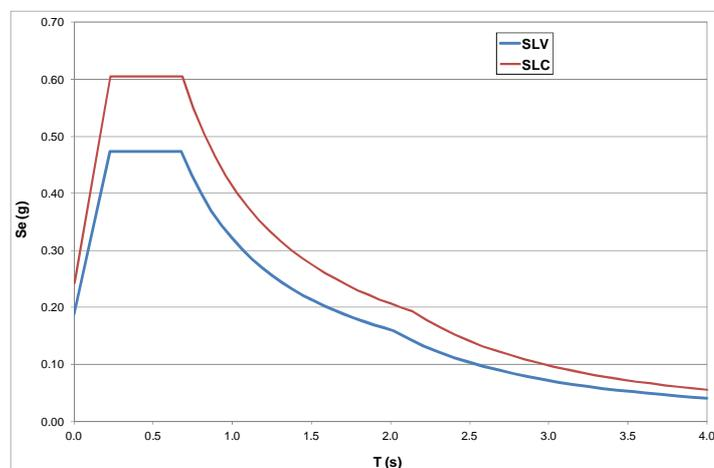
**Figure 2.** Comparison of elastic response spectrum for the structure (SLV) and for the seismic isolation system (SLC) of the Bridge over the Po river in Piacenza.
