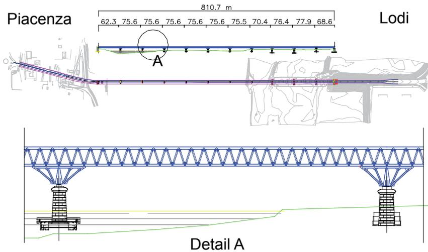
**Figure 1.** Elevation of the main bridge, alignment and span detail (Unit: m).
