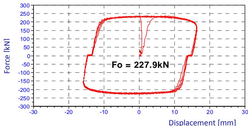
**Figure 7.** Force vs. displacement graph obtained in dynamic test on a viscous damper characterised by maximum force 250 kN and maximum stroke  $\pm 75$  mm (maximum velocity 150 mm/s).
