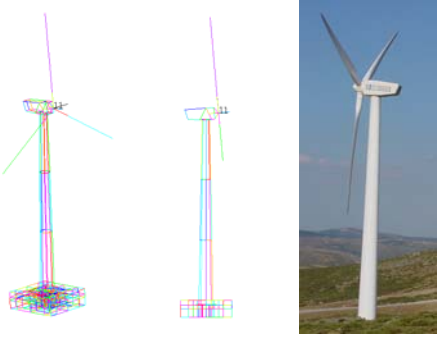
Figure 5. Wireframe model and photograph of the wind turbine MADE AE-46/1
