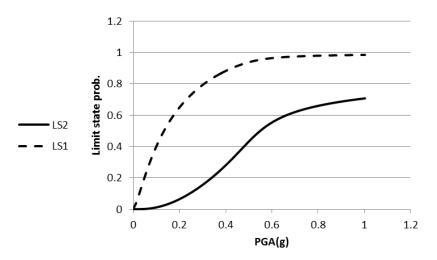
Figure 2.7. Fragility curves (LS1=Elastic limit strength, LS2=Maximum strength)
