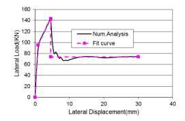
Figure 1.1. A sample of the lateral force-displacement curves of confined masonry walls (Ranjbaran et al. 2012)
