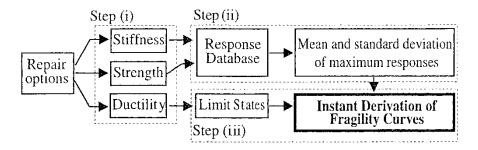
Figure 2.1. Overal procedure of the parameterized fragility curves (Jeong and Elnashai, 2007)
