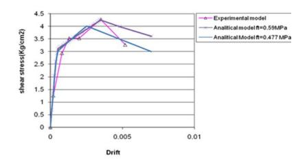
Figure 1.2. Comparison of capacity curves obtained by experimental and numerical model (Ranjbaran et al. 2012
