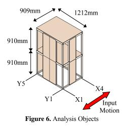
for 1F story stiffness (k1). In this study, k2/k1 assumed it k2/k1=0.8,0.6. When k2/k1 was changed, k1 was not changed but k2 was changed. The other is the ratio (m2/m1) of 2F story's mass (m2) for 1F story's mass (m1). In this study, m2/m1 assumed it m2/m1=0.9,0.6. When m2/m1 was changed, total mass (m1+m2) was not changed. Total mass assumed it 360kg in reference to [3] and [4].
