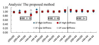
Figure 20. The Accuracy of The Proposed Method (The Maximum Response)
