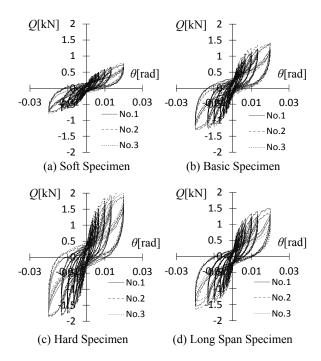
**Figure 4.** Results of Shear Wall Tests (Q- $\theta$ )
