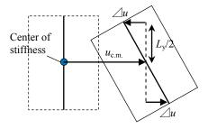
**Figure 13.** The Response Rate of Twist ( $\Delta u/u_{c.m.}$ )
