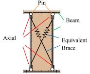
Figure 9. Frame Model of Shear Wall
