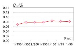
**Figure 5.** The Comparison of Shear Force of Each Deformation Angle (Q<sub>1/3</sub>/Q<sub>f</sub>)
