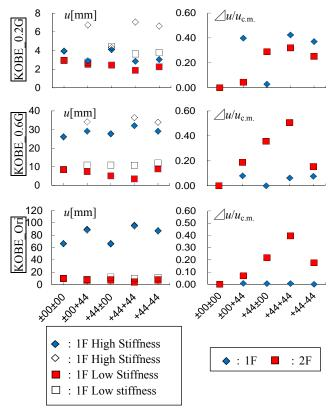
**Figure 11.** The Maximum Displacement of Each Wall
