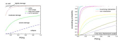
Figure 4. Seismic Vulnerability Curves
