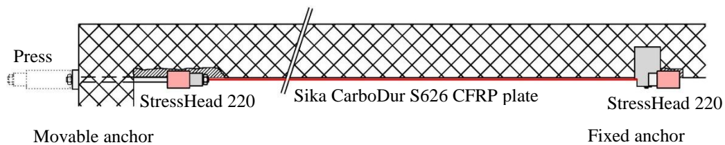
Figure 4: Schematic drawing of the StressHead CarboStress post-tensioning system
