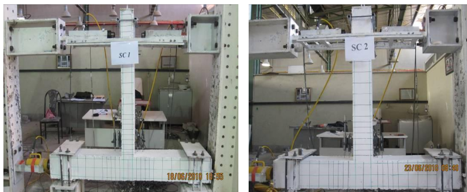
Figure 1. Joints specimens of SC1&SC2 before loading
