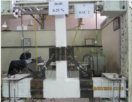
Figure 3. Retrofitted specimen RSC1 before testing
