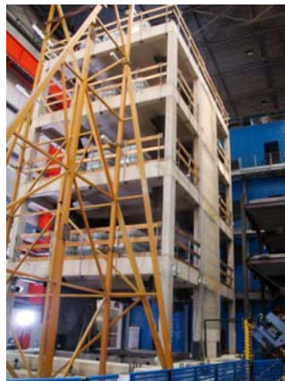
Figure 2.3. Elevation of the specimen in the lab. The wall shown on the right of the picture is the south wall and the one on the background is the north wall
