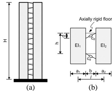
**Figure 2.1.** Structural systems considered in the study: a) viscously coupled shear walls, and b) parameters of the viscously coupled shear walls.
