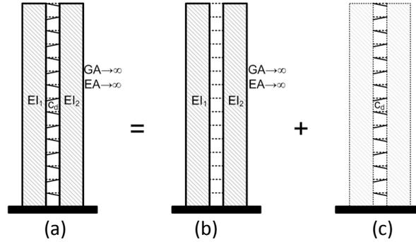
**Figure 2.2.** Partitioning of the total structural system (a) to its two parallel components: the “stiffness system” that resists displacements and deforms in bending (b), and the “damping system” that resists velocities where the deformations are concentrated in the dampers (c).
