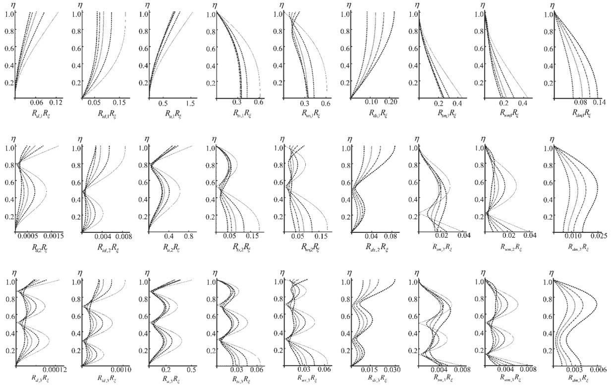
**Figure 6.1.**  $R$  coefficients multiplied by  $R_\xi$  for various responses (columns) for the first three modes (rows) using various damping values ( $\xi=0$  continuous,  $\xi=0.1$  dashed,  $\xi=0.2$  dotted,  $\xi=0.3$  dashed-dotted,  $\xi=0.4$  dashed thick).
