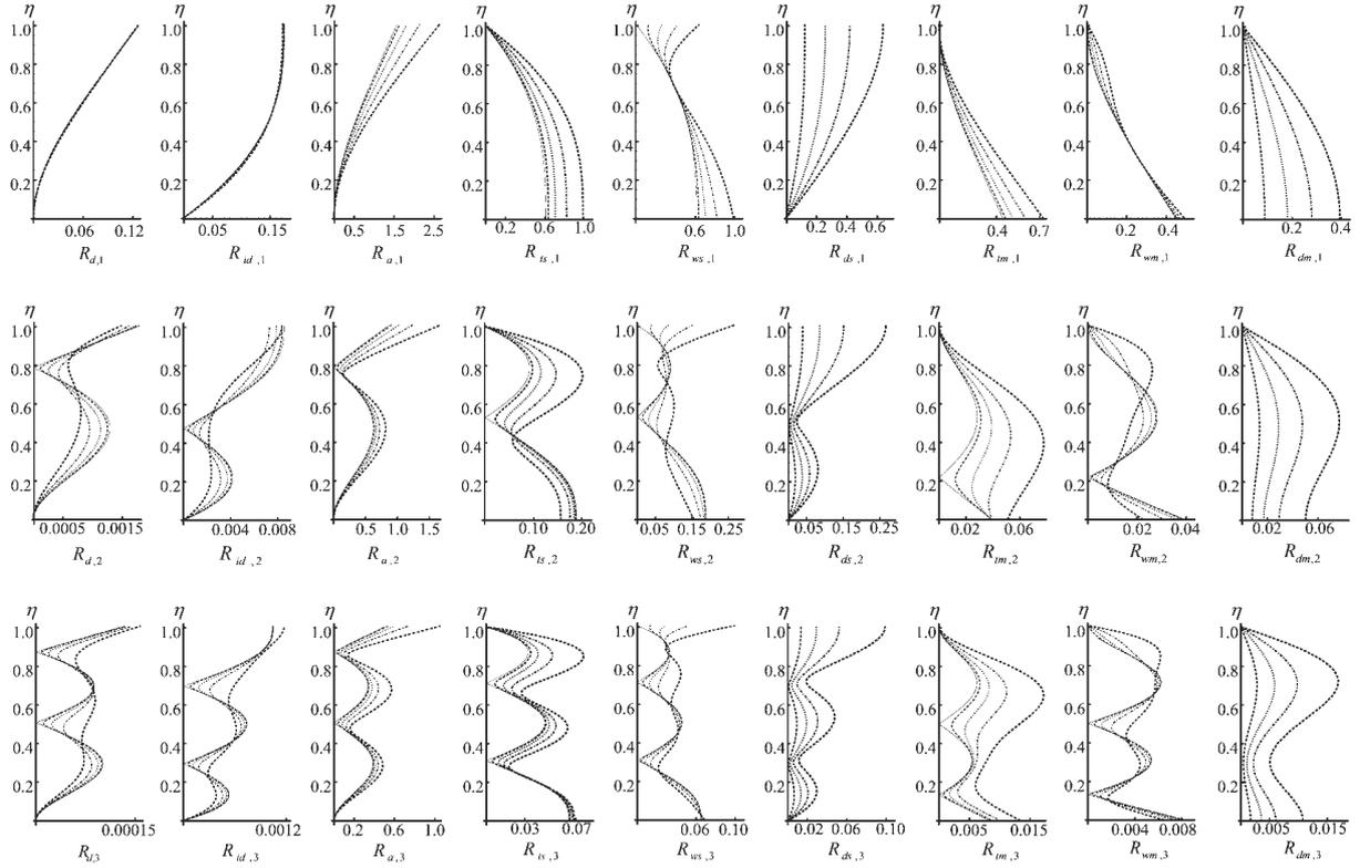
**Figure 5.1.**  $R$  coefficients for various responses (columns) for the first three modes (rows) using various damping values ( $\xi=0$  continuous,  $\xi=0.1$  dashed,  $\xi=0.2$  dotted,  $\xi=0.3$  dashed-dotted,  $\xi=0.4$  dashed thick).
