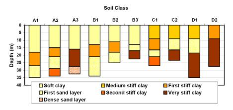
Figure 4.3. Generalized Soil Profiles in the Study Area
