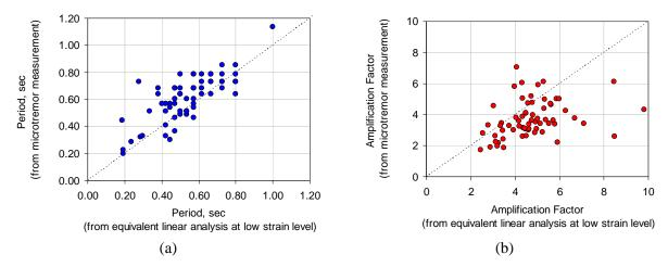
Figure 5.1. Comparison of results from microtremor measurements and linear analysis; (a) Predominant period and (b) Amplification factor.
