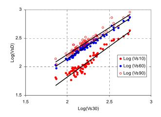
Figure 4.6. Relations among  $V_{S30}$  and  $V_{S10}$ ,  $V_{S60}$ ,  $V_{S90}$
