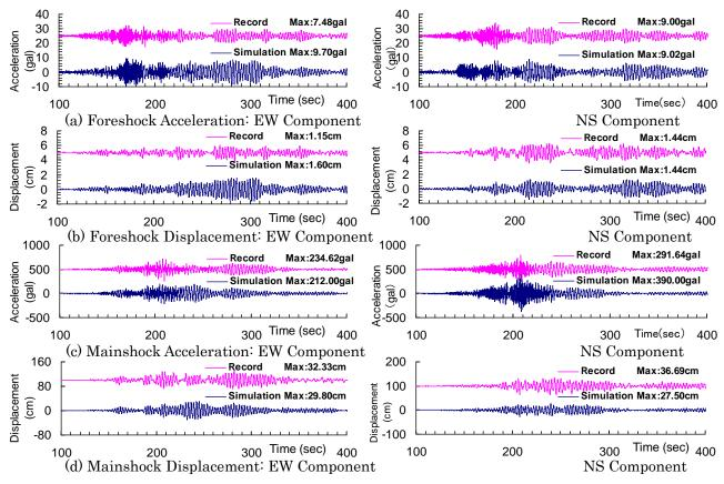
Figure 10. Observed and simulated accelerations and displacements of the 29th floor for the fore- and main-shocks
