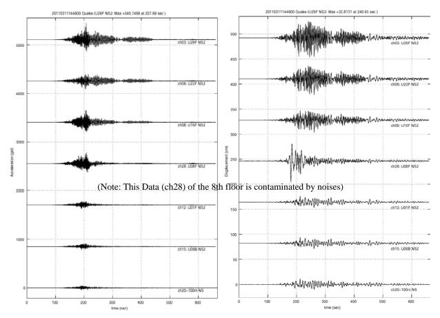
Figure 5. Accelerations (left) and displacements (right) of NS components from GL-100 m to the Top Floor
