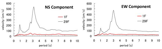
Figure 7. Velocity response spectra (h=5%) of the campus building of Kogakuin University
