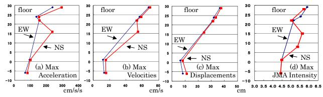
Figure 6. Maximum Accelerations, Velocities, Displacements, and the JMA Intensities of Kogakuin University.
