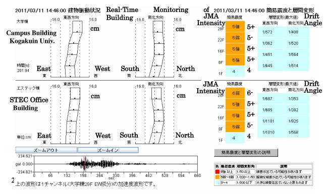
Figure 12. RMS (Real-Time Strong Motion Monitoring System) after the 2012 East Japan earthquake at Kogakuin University
