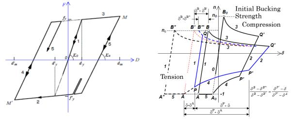
Figure 9. Non-linear hysteretic models for beams and braces of the 3D structural model of Kogakuin University
