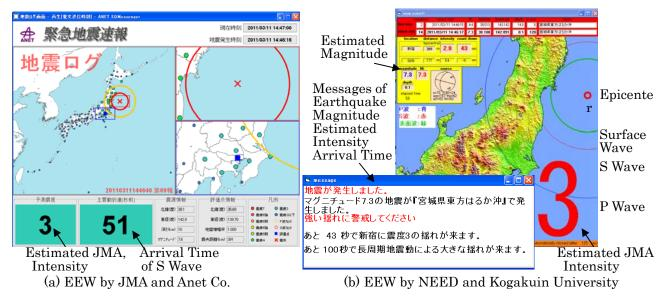
Figure 11. EEW (Earthquake Early Warning System) after the 2012 East Japan earthquake at Kogakuin University
