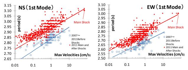
Figure 8. Dependency of natural periods on the maximum velocities of the 29th floor of the university building
