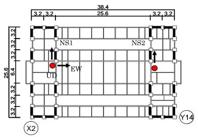
Figure 2. Structural plan and location of strong motion seismometers
