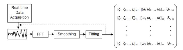
Figure 4. Real-time power spectral model
