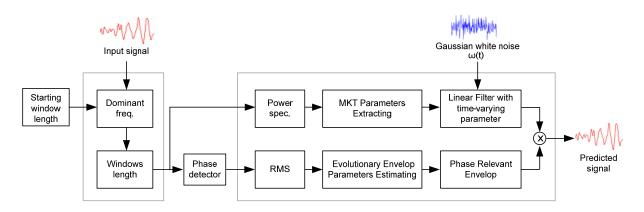
Figure 1. Schematic of the real-time stochastic prediction model
