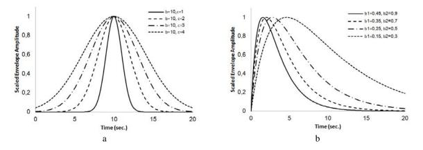
Figure 3. a) Gaussian envelope function for b=10 and various c, b) Shinozuka-Sato envelope function for various  $b_1$  and  $b_2$
