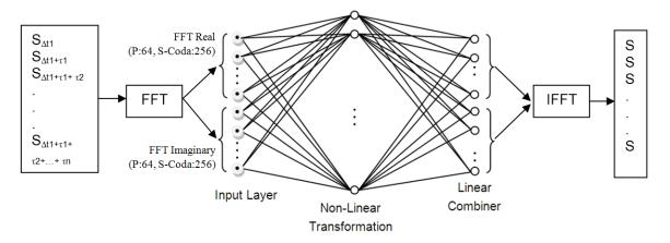
Figure 7. Architecture of amplitude evolutionary Artificial Neural Networks (AE-ANNs)
