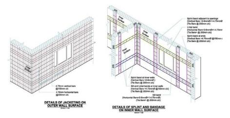
Figure 2. Typical design of proposed retrofitting (source NSET)
