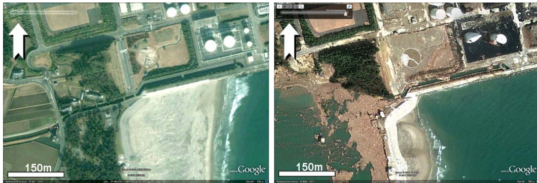
Figure 1. Minamisoma coastal area (Fukushima prefecture). Total erosion of shoreline, total deforestation of vegetation in low lying area, submergence of low lying cultivated area into a lagoon-like form, functioning as a retention pond for water backwash after the tsunami. Debris accumulated behind the road embankment and into the newly formed lagoon. Treatment Plant in nearby industry is devastated, as much as the tanks which may also have been set on fire during the disaster.
