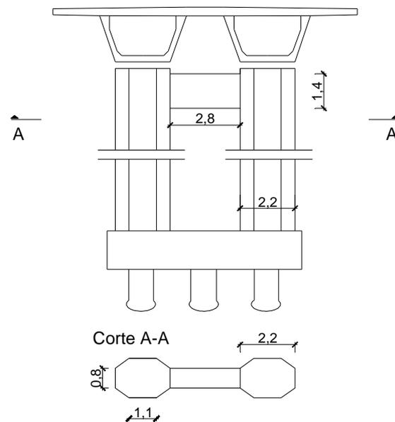
**Figure 1.** Geometrical configuration of the studied bent-type frame
