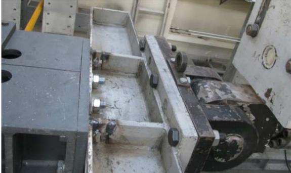
**Figure 6.** Load distribution system
