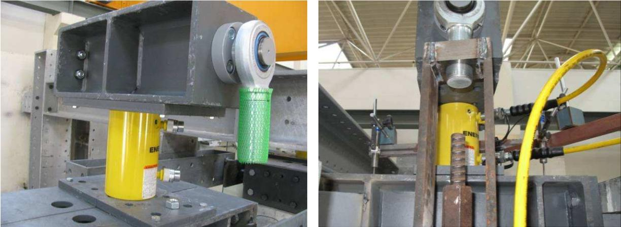
**Figure 5.** Constant axial load control system (jack, hinges and Dywidag rods)
