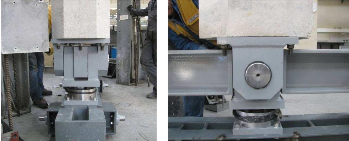
**Figure 8.** Column base hinge mechanism
