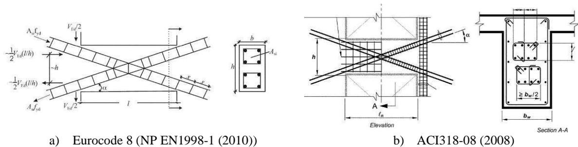
Figure 2. Diagonal reinforcement layout for coupling beams
