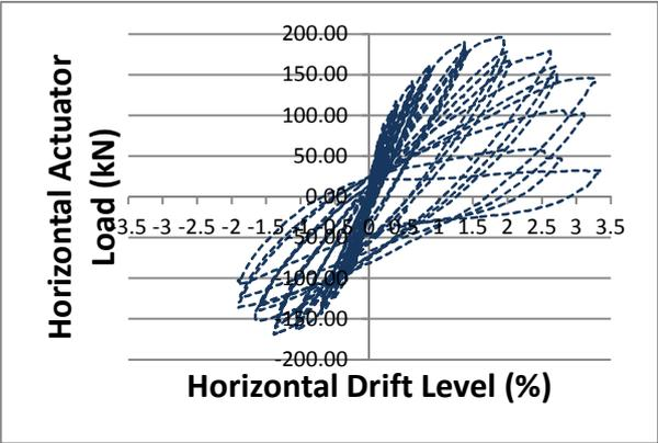
**Figure 10.** Force – drift curve for SP\_M01 test.
