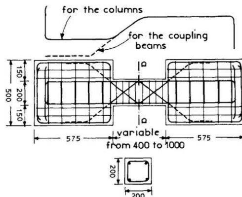
Figure 3. Rhombic truss reinforcement layout (Tegos and Penelis (1988))
