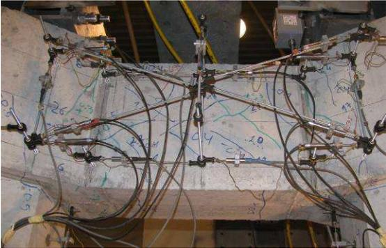
a) Cracking pattern – 0.75%
