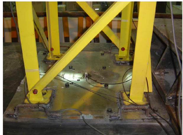
Figure 8. the position of transducer on base plate
