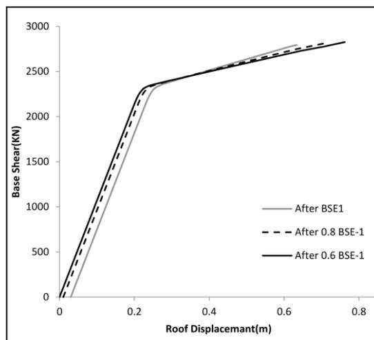
**Figure 4.2.** Capacity Curves after 3 assumed earthquakes
