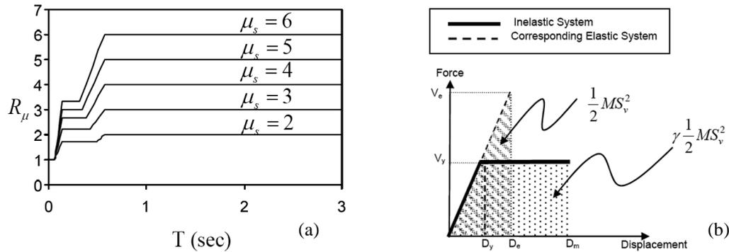
**Figure 2.1.** (a) Plot of Newmark and Hall's Equations (Liao, 2010). (b) Modified Energy Balance Concept (Liao, 2010).
