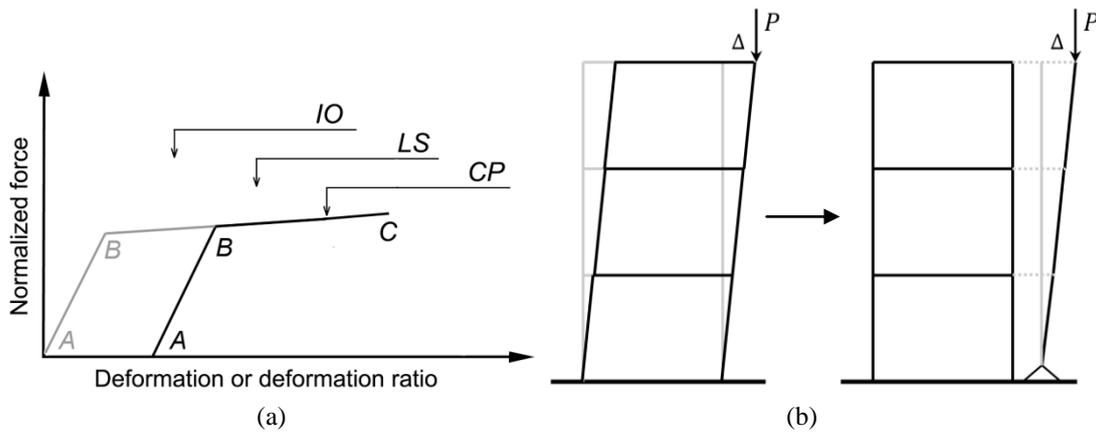
**Figure 3.1.** (a) Changing in Plastic hinge after an earthquake. (b) Inclined leaning column for considering initial P- $\Delta$  effects
