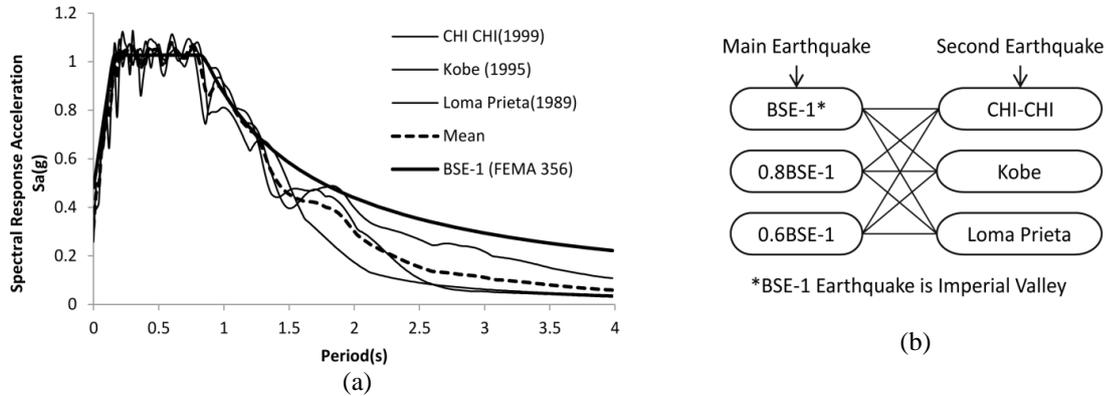
Figure 5.1. (a) Three records scaled in BSE-1 Spectrum as second earthquakes. (b) Consecutive Nonlinear Dynamic Analysis.
