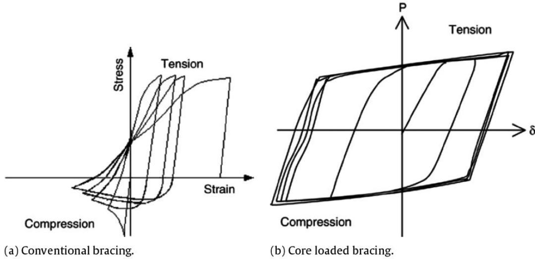
**Figure 1.1.** Difference in energy dissipation between conventional braces and BRBs under cyclic loading.(Mahmoudi, 2010)
