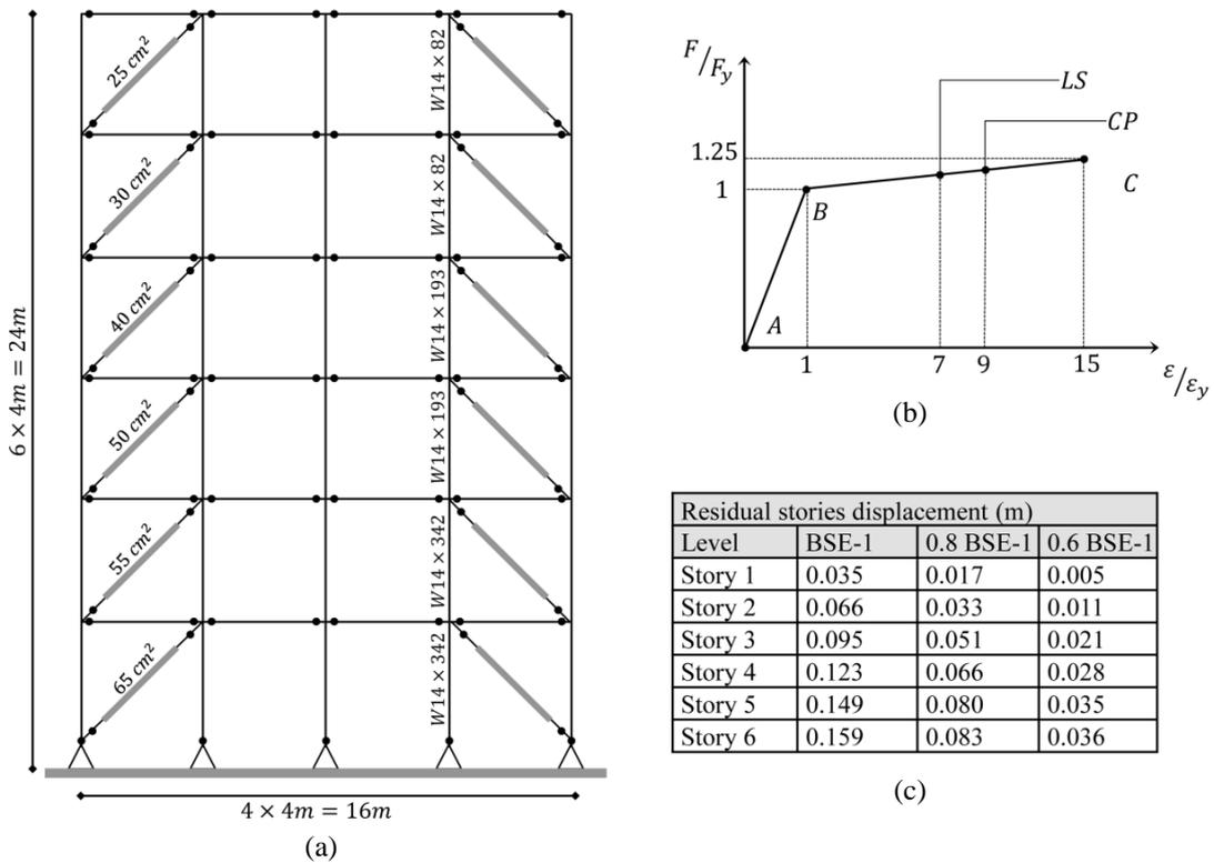
**Figure 4.1.** (a) Configuration of six stories BRBF model. (b) Nonlinear Steel01 material in OPENSEES (c) Residual displacement for each earthquake
