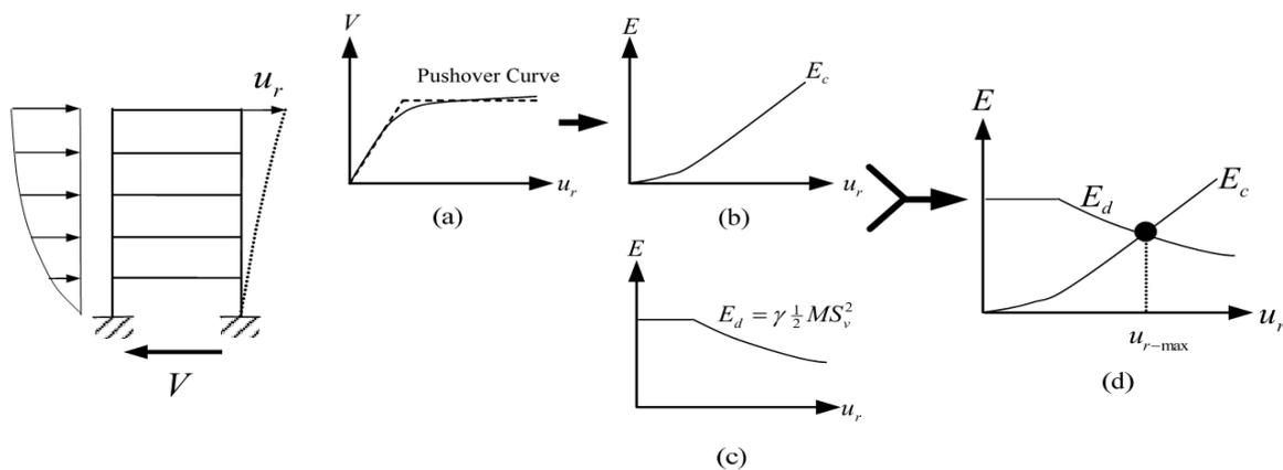
**Figure 2.2.** General procedure of energy balance concept for Target displacement evaluation (Liao, 2010).
