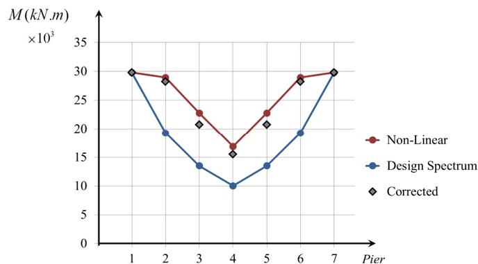
Figure 10. Comparison of the bending moments obtained with different methodologies
