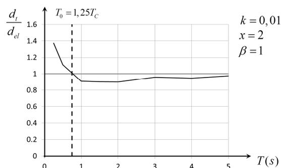
**Figure 8.** Normalised displacement as a function of  $T$  ( $k=0,01$ ;  $x=2$ ;  $\beta=1$ )
