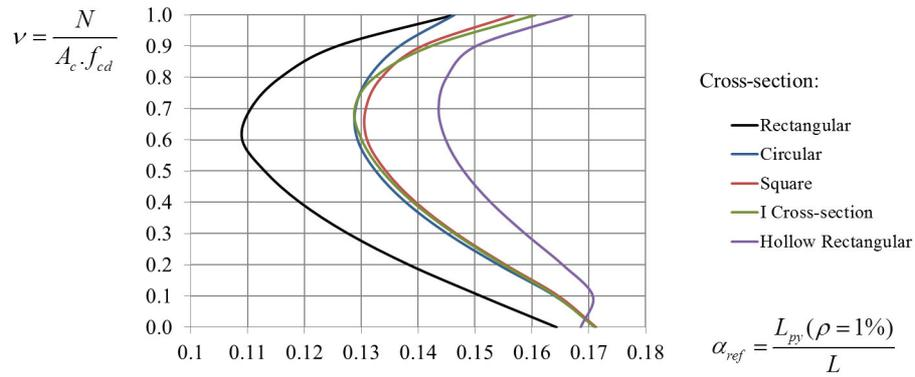
**Figure 3.** Value of  $\alpha_{ref}$  as a function of  $v$  for several cross-section types
