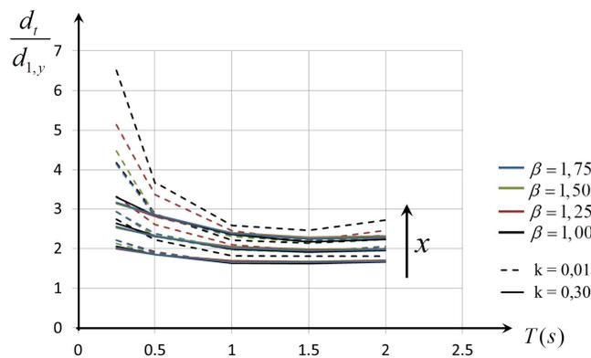
**Figure 6.** Demanded ductility in pier 1 as a function of  $T$ .
