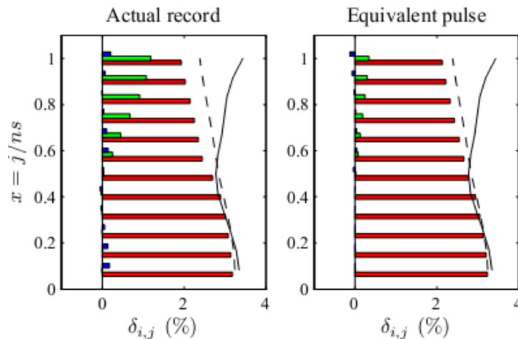
**Figure 2.** IDR along the dimensionless height of the 12-story SMRF subjected to the ground motion and its equivalent pulse shown in Fig. 1. The red, green, and blue bars represent the contributions of the first, second, and third modes respectively. Maximum interstory drifts considering all modes of vibration are shown with the solid (for actual record) and dashed (for equivalent pulse) lines.
