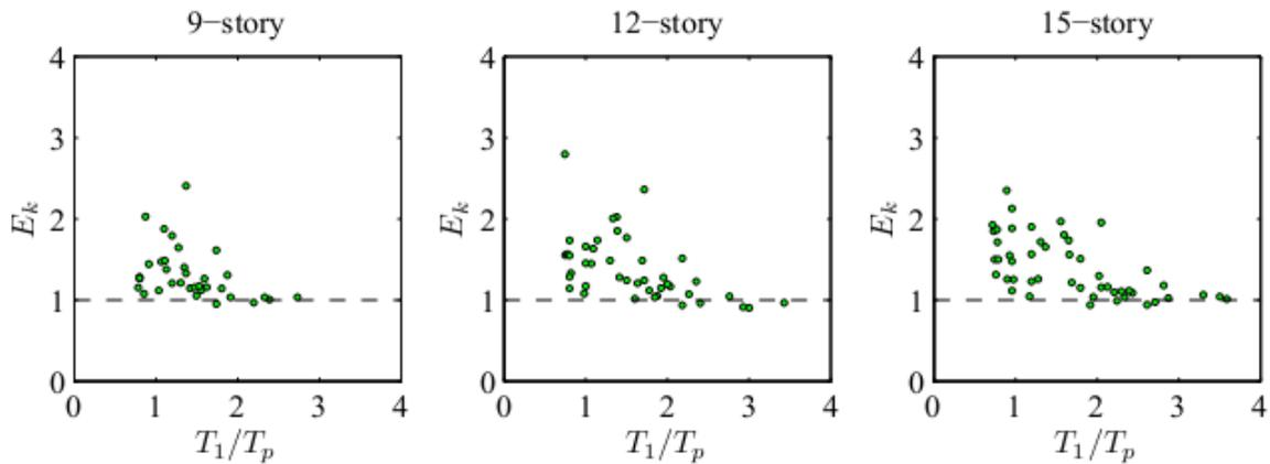
**Figure 3.** Errors in the computation of interstory drift ratio at the roof of 9-, 12-, and 15-story SMRF due to the use of an equivalent pulse instead of an actual ground-motion record.
