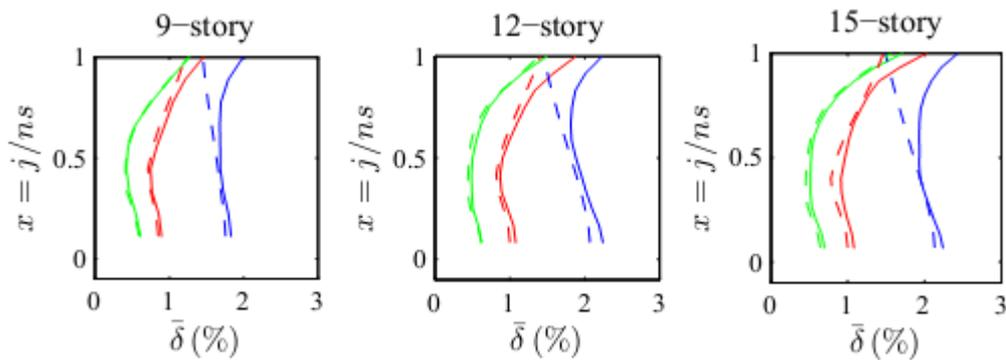
**Figure 4.** Mean interstorey drifts of the 9-, 12-, and 15 -story SMRF. The solid and the dashed lines represent the results obtained by using the actual records and their equivalent pulses respectively. Blue, red, and green lines correspond to  $0.7T_p \leq T_1 < 1.3T_p$ ,  $1.3T_p \leq T_1 < 2.0T_p$ , and  $2.0T_p \leq T_1$ , respectively.
