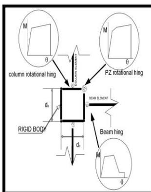
Figure 15. PZ modeling detailing
