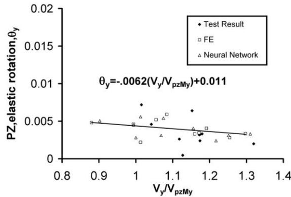
**Figure 10.** PZ plastic rotation versus  $V_y/V_{PZM_y}$  for (WUF) connection
