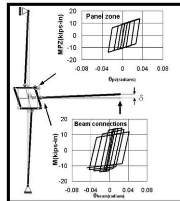
Figure 17. Results for the analytical model (UCB-AN1)
