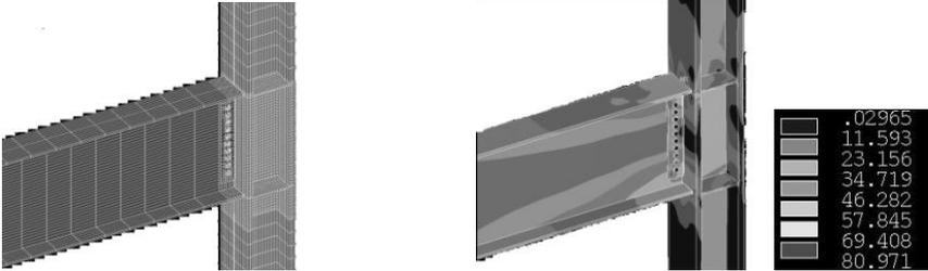
Figure 6. FE modeling of connection (RFSPN1) Figure 7. Von Mises distribution of connection (RFSPN1)
