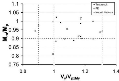
**Figure 8.** Moment ratio ( $M_m/M_p$ ) versus  $V_y/V_{PZM_y}$  for (WUF)
