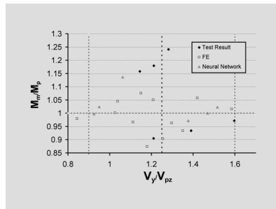
**Figure 11.** FE model of Specimen (RFSAN1) **Figure 12.** Moment ratio ( $M_m/M_p$ ) versus  $V_y/V_{PZM_y}$
