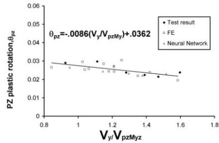
Figure 14. PZ plastic rotation versus  $V_y/V_{pzM_y}$
