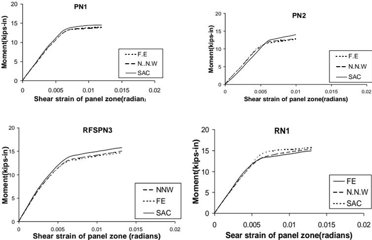
Figure 5. Comparison between result of FE and N.N.W and experimental result for (WUF-B) connection
