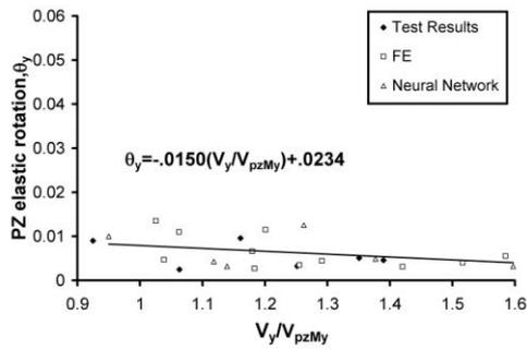
Figure 13. PZ elastic rotation versus  $V_y/V_{pzM_y}$
