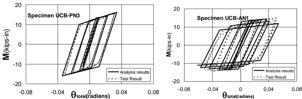
**Figure 18.** Total rotation versus total moment of test and analysis result for test specimen UCB-PN3 (test specimen with WUF-B) and UCB-AN1 (test specimen with cover plate connection)
