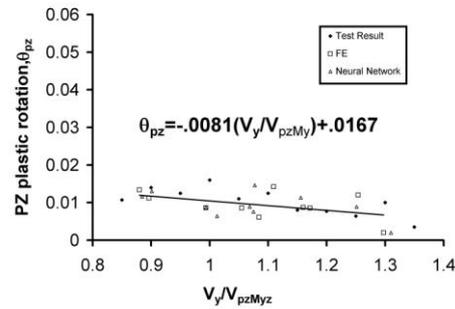
**Figure 9.** PZ plastic rotation versus  $V_y/V_{PZM_y}$  for (WUF) connection connection
