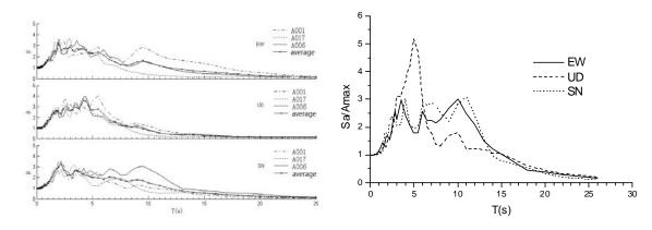
Figure 3 Acceleration response spectra of bedrock site
