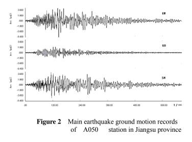
valuable to study of long-period seismic ground motion and aseismic design of long-period structures.
