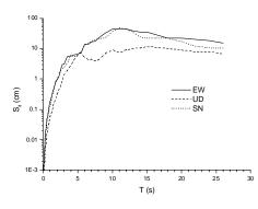
**Figure 6** Displacement response spectra of ground motion records (A050, damping ratio: 0.05)
