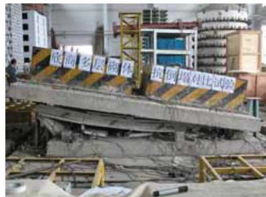
(b) Totally collapsed after 0.6g
