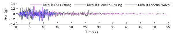
Figure 4.5. Modified time-acceleration curves of selected seismic waves
