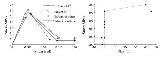
Figure 4.2. Shear stress-strain of joints
