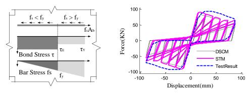
Figure 3.3. Distribution of steel stress and bond stress in the joint panel
