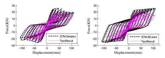
Figure 3.7. Hysteretic curves of analytical model and experiment
