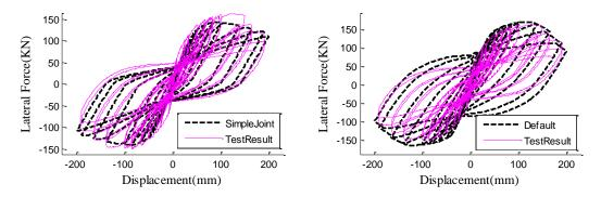
Figure 3.9. Hysteretic curves of the model SimpleJoint and experiment
