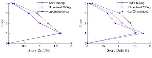
Figure 4.7. Distribution of maximum story drift with SimpleJoint
