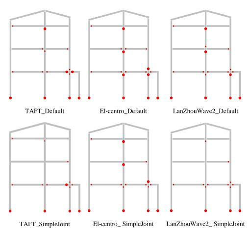
Figure 4.9. Failure modes of structure with two modeling methods under selected waves
