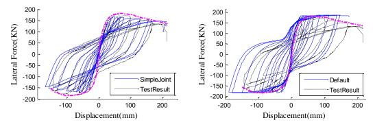
Figure 3.8. Hysteretic curves of the model with SimpleJoint and experiment
