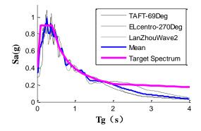
Figure 4.4. Modified response spectrum of selected earthquake waves compared with the target one
