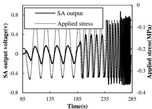
**Figure 4.3.** Frequency sweep loading scheme
