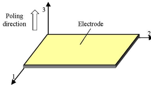
**Figure 1.1.** PZT patch and poling direction
