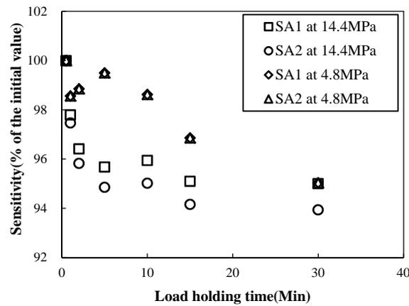
**Figure 4.8.** Sensitivity variation of SA vs. holding time
