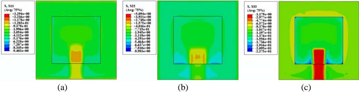
Figure 3.2. Stress distribution in the mid interface of the smart aggregate in the: (a)1 direction, (b) 2 direction and (c) 3 direction.
