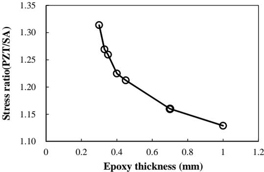
Figure 3.3. Stress ratio (PZT/SA) vs. epoxy thickness
