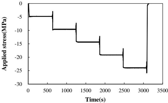
Figure 4.9. The applied stress for evaluating the influence of pre-stress
