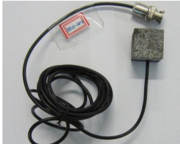
**Figure 3.1.** Structure of the proposed smart aggregate
