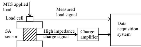
**Figure 4.1.** Test configuration of the test system
