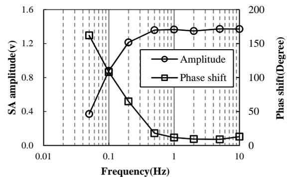
**Figure 4.4.** Frequency response of both amplitude and the phase shift of the smart aggregate
