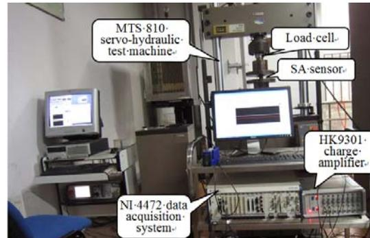
**Figure 4.2.** Picture of the test system
