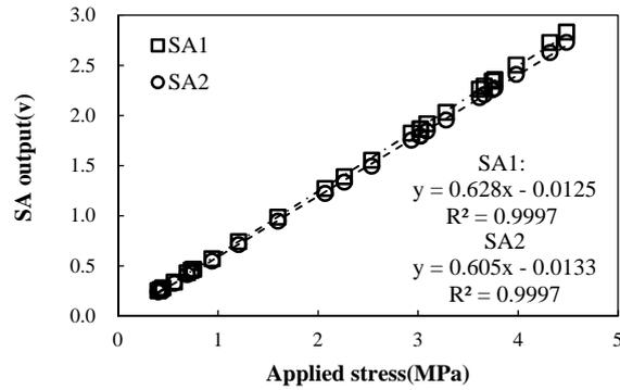
**Figure 4.7.** Amplitudes of smart aggregate output vs. applied stress during 994-1006s
