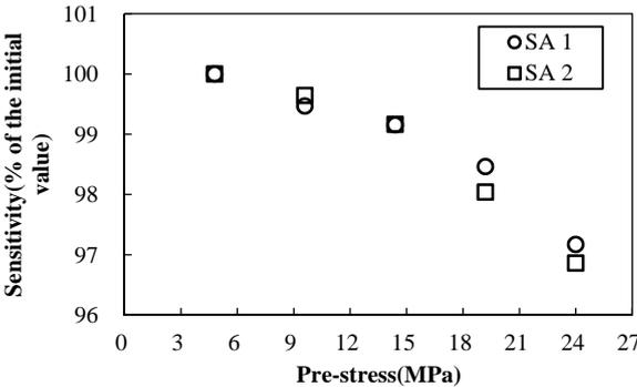
Figure 4.11. Smart aggregate sensitivity vs. pre-stress
