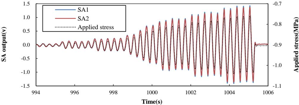
Figure 4.6. The applied sine stress waves and the smart aggregate output during 994-1006s
