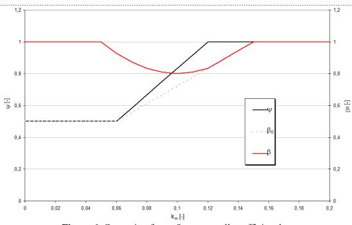
Figure 6. Correction factor  $\beta$  versus wall coefficient  $k_w$
