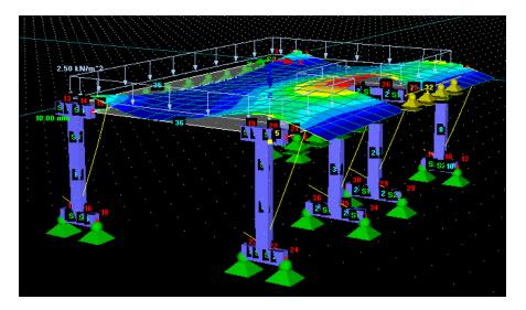
Figure 9. Isometric view of one story finite element model for a terraced house
