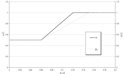
**Figure 5.** Dependency of fixture degree  $\psi$  and coefficient of clamping efficiency  $\beta_0$  from wall coefficient k<sub>w</sub>
