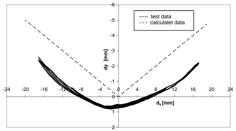
**Figure 2.** "Growth" of a shear wall due to lateral deflection from experiment LAC-dm-125-110-1 after Fehling et al. (2008a)
