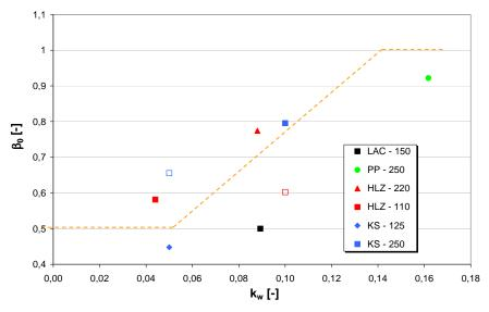
Figure 4. Influence of wall coefficient  $k_w$  on the coefficient of clamping efficiency  $\beta_0$
