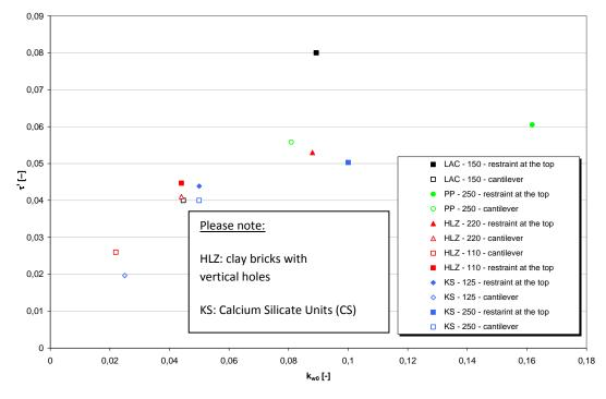
Figure 3. Influence of moment fixture (clamping) on the non-dimensional shear capacity
