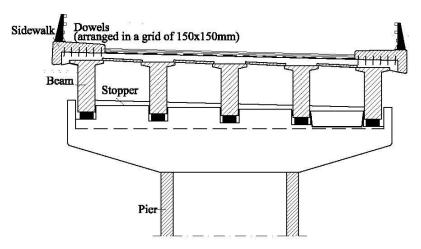
Figure 2.3. Cross-section of the sidewalk-restrainers at the anchorage length (Section A-A in Fig. 2.1)
