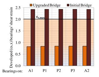
Figure 3.6. The values of the allowable ( $\varepsilon_{s,max}$ ) and the developed ( $\varepsilon_{s,x}$ ) shear strains of the elastomeric bearing for the longitudinal design earthquake ( $a_g=0.24g$ )
