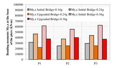
Figure 3.4. The moment actions  $(M_{y,x})$  at the base of the piers for the longitudinal design earthquake (ground acceleration 0.16g, 0.24g and 0.36)
