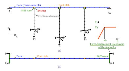
Figure 3.3. The model of the upgraded bridge: (a) Longitudinal section and (b) Plan view
