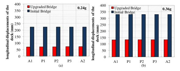
Figure 3.5. The longitudinal displacements of the deck over the piers (a)  $a_g=0.24g$  and (b)  $a_g=0.36g$
