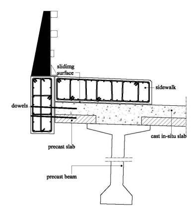
Figure 2.2. Cross-section of the sidewalks-restrainers (section B-B in Fig.2.1)
