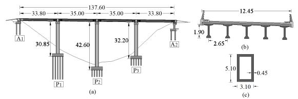
Figure 3.1. The "reference" bridge (a) Longitudinal section, (b) Cross –section of the deck and (c) Cross – section of the piers
