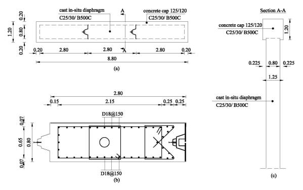
Figure 3.2. (a) Plan view of the barrette wall (b) reinforcement detailing and (c) Section A-A
