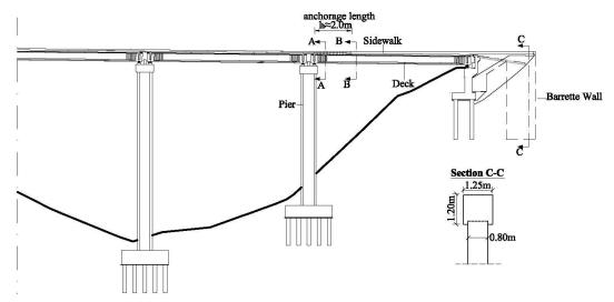
Figure 2.1. Longitudinal section of a precast I-beam bridge in which the proposed sidewalks-restrainers are implemented
