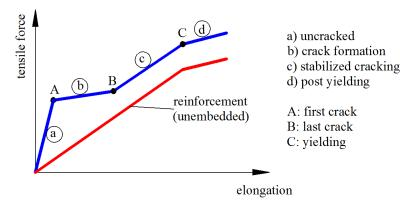
Figure 2.4. Idealized behaviour of a reinforced concrete tie
