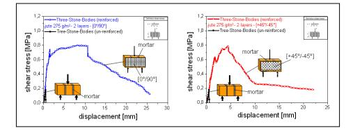
**Figure 7.** Graphs of mean values of shear strength - joint displacement, left: Comparison of Three-Stone-Bodies with and without reinforcement and fibre orientation of  $[0^{\circ}/90^{\circ}]$ , right: Comparison of Three-Stone-Bodies with and without reinforcement and fibre orientation of  $[+45^{\circ}/-45^{\circ}]$
