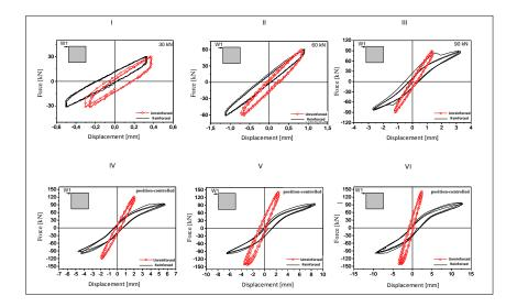
Figure 12. Horizontal Force-Displacement behaviour of reinforced in comparison to unreinforced wall
