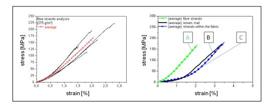
**Figure 2**. Test of single fibre strands (left), Comparison of stress-strain behaviour of single jute fibre strands (right), fibre mats and single strands within a mat (jute mat - 275 g/m<sup>2</sup>)
