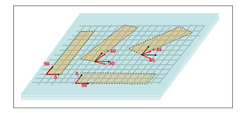
Figure 3. Schematic illustration of test strips for the determination of mechanical properties
