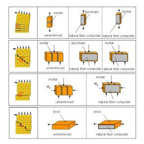
Figure 5. Different models of small masonry for the simulation of wear resulting from forces within the plane of the masonry with and without reinforcement
