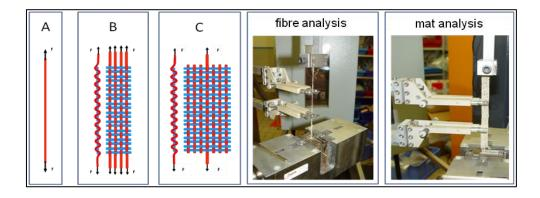
Figure 1. Investigations of single jute fibre strands, fibre mats and single strands within a mat
