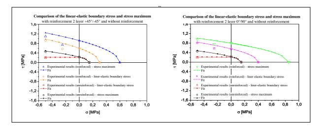
**Figure 9.** Comparison of the linear-elastic boundary stress and stress maximum for unreinforced and reinforced sample with 2 layers - Left: fibre orientation of [+45°/-45°], right: fibre orientation of [0°/90°]
