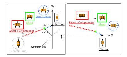
Figure 8. Representation of the experimental results in main-stress and  $\tau$ - $\sigma$ -diagram for liner-elastic boundary stress and stress maximum
