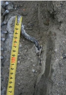
Figure 4.2 : Cut of jacketed specimen 14 after loading- dowel deformation
