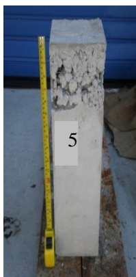
Figure 2.1. Specimen with construction (initial) damages
