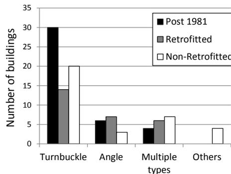
**Figure 2.4.** Section shape of the roof braces
