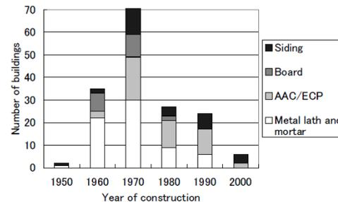
**Figure 3.4.** Distribution of the types of exterior walls grouped by the year of construction
