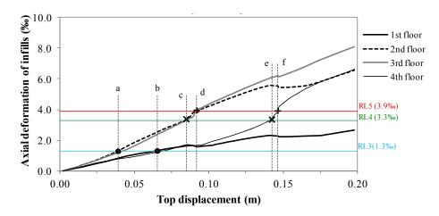
Figure 9. Local inelastic responses of the infill panels of the fully infilled 6-story frame structure with equal interstory heights.
