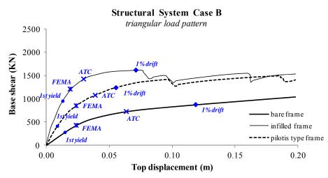
Figure 4. Capacity curves of the 6-story frame structures with the height at the base to be greater than the other equal interstory heights (Case B).
