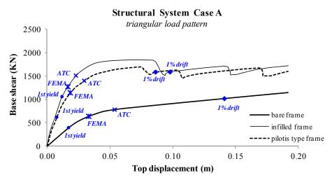
Figure 3. Capacity curves of the 6-story frame structures with equal interstory heights.
