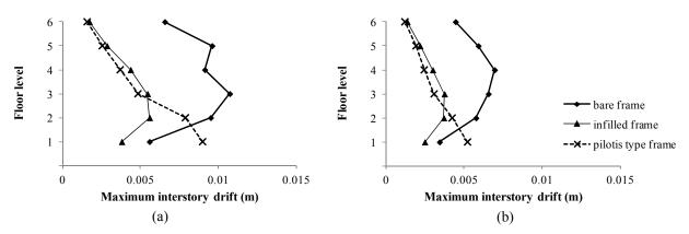
**Figure 6.** Maximum interstory drifts of the 6-story frame structures with equal interstory heights (Case A): a) at performance points to ATC40 and b) at target displacement to FEMA356.
