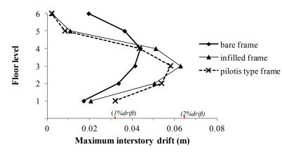
Figure 5. Maximum interstory drifts of the 6-story frame structures with equal interstory heights (Case A) at top drift equal to 1%h<sub>str</sub>.
