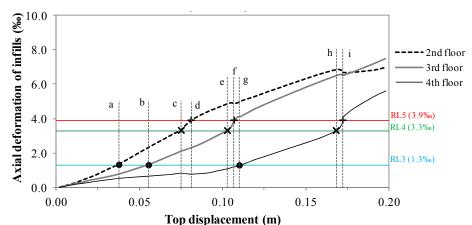
Figure 10. Local inelastic responses of the infill panels of the pilotis type 6-story frame structure with equal interstory heights.
