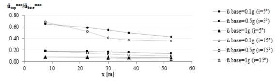
Figure 3.3. Amplification factors of model 2 - Vs<sub>1</sub>/Vs<sub>2</sub>=2.
