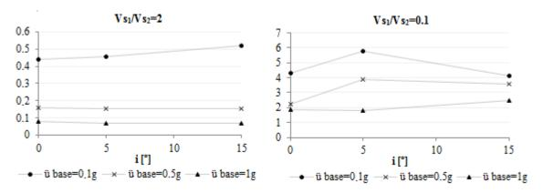
Figure 3.7. Amplification factors dependence on the inclination of the interface, i.
