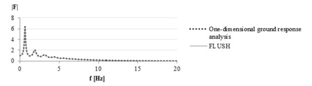
Figure 2.2. Transfer functions: model response (FLUSH) vs. vertically propagating shear waves in elastic damped layer.
