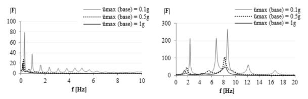
Figure 3.2. Transfer functions obtained with models with  $h_1=10m$  and  $h_2=30m$ , for  $Vs_1/Vs_2=2$  (left) and  $Vs_1/Vs_2=0.1$  (right).
