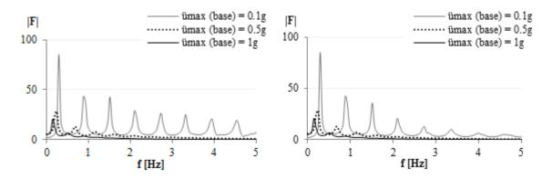
**Figure 3.5.** Amplification factors of model 2.1.1(i=5° and Vs<sub>1</sub>/Vs<sub>2</sub>=0.1), located at 7.5 m distance (1<sup>st</sup> point; left) and at 52.5 m (5<sup>th</sup> point; right). See Fig. 3.7 for location of the points.
