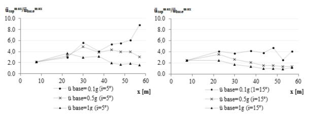
Figure 3.4. Amplification factors of model 2 - Vs<sub>1</sub>/Vs<sub>2</sub>=0.1.
