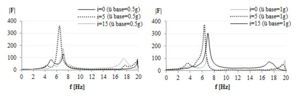
Figure 3.9. Transfer functions associated to the control point ( $h_1$ =3m and  $h_2$ =37m) for Vs<sub>1</sub>/Vs<sub>2</sub>=0.1.
