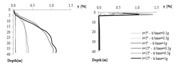
**Figure 3.10.** Strain profiles of the models with  $Vs_1/Vs_2=2$  (left) and  $Vs_1/Vs_2=0.1$  (right) (h<sub>1</sub>=3m and h<sub>2</sub>=37m).
