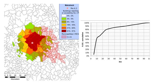
**Figure 2.2**. Damage scenario calculated with the CF on soil, expressed as percentage of buildings reaching or exceeding SL1 (left) in each municipality. On the right the cumulative distribution of the percentage of buildings reaching or exceeding SL1 with respect to the total damage within 100 km from the epicentre
