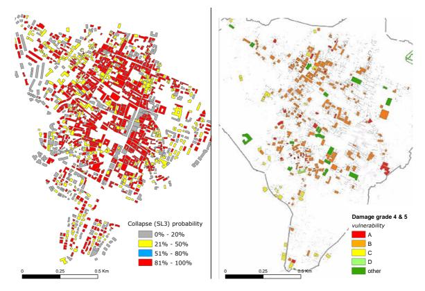
**Figure 3.4**. Left, damage scenario expressed in terms of probability of reaching the limit state of collapse (SL3), with site effects from the microzonation study. Right, the real damage data showing the buildings experiencing damage grade 4 and 5, classified by vulnerability class (modified bye Tertulliani et al., 2011).
