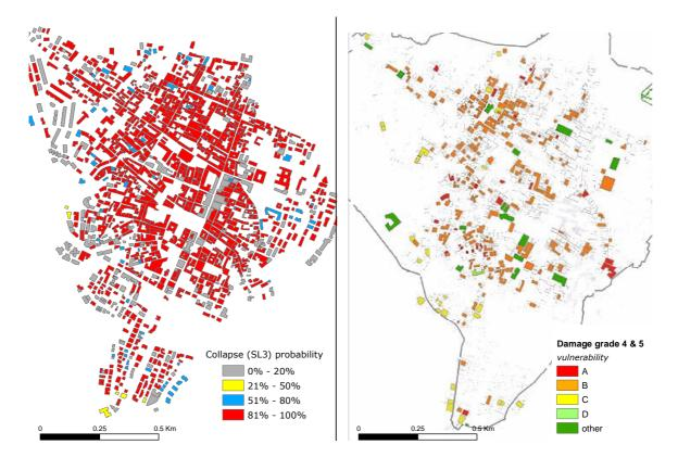
**Figura 3.3.** Left, damage scenario expressed in terms of probability of reaching the limit state of collapse (SL3), with site effects from the national soil map. Right, the real damage data showing the buildings experiencing damage grade 4 and 5, classified by vulnerability class (modified bye Tertulliani et al., 2011).
