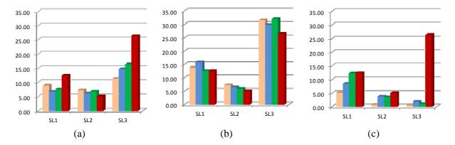
**Figure 2.4.** Results of scenarios obtained with three GMPEs using the median (a), +1STD (b), -1STD (c) compared with the real data for the municipalities with I >=6, expressed as percentage of buildings experiencing the damage states SL1, Sl2 and SL3. Pink = CF, Blue = AB, Green = SP, Red = real data.
