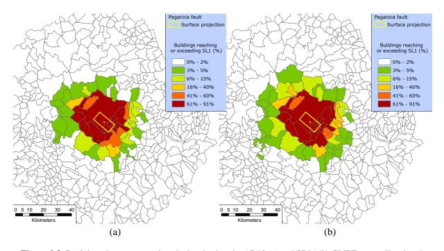
**Figure 2.3.** Real time damage scenario calculated using the AB10 (a) and SP96 (b) GMPEs, on soil and rock respectively, using the distance from the surface projection of the Paganica fault, recognised as the source of the L'Aquila 2009 earthquake
