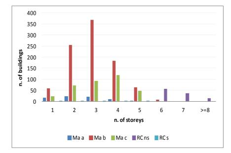
**Figure 3.1.** Building distribution in vulnerability classes and number of storeys for the L'Aquila historical centre. "Ma a" = Masonry - high vulnerability, "Ma b" = Masonry - average vulnerability, "Ma c = Masonry - low vulnerability", "RC ns" = Reinforced Concrete not seismically designed, "RC s" = Reinforced Concrete seismically designed.
