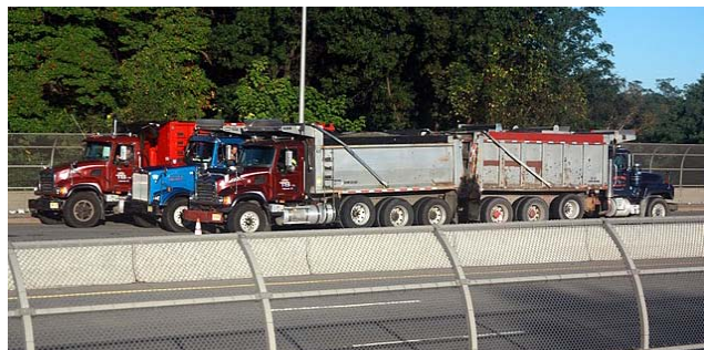
Figure 5. Picture for six truck load test on Southbound Span 2
