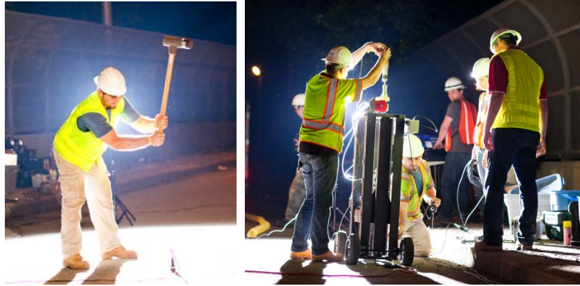
Figure 4. Excitation by (a) Sledge hammer (b) Drexel drop hammer
