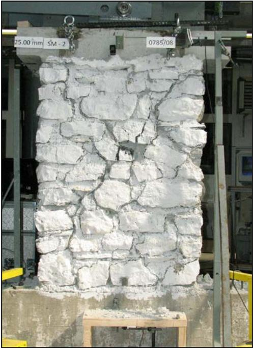
Figure 5. Control wall: damage at ultimate state
