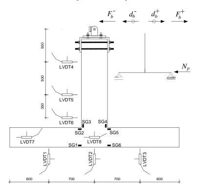
Figure 2.3. Instrumentation. Note: all units in millimeters
