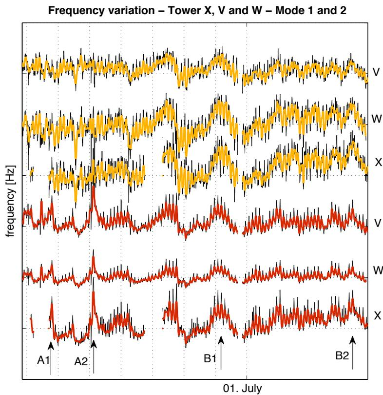
**Figure 4.** Frequency variations (black lines) for the three towers considering the first (bending, yellow line) and second (torsion, red line) modes. Thick lines correspond to the smoothed variation, computed as the mean value of the frequency within a sliding window (5 hours length). Value (Y-axis) are in Hz.
