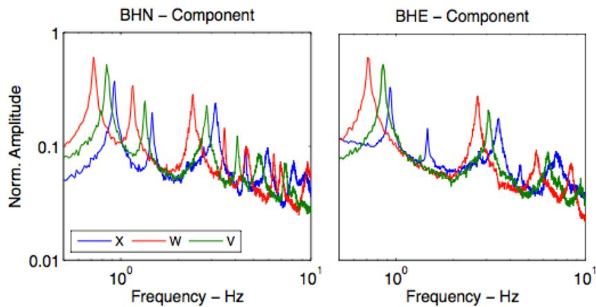
**Figure 2.** Average normalised amplitude of the Fourier transform computed on one ambient vibrations recording (one hour length) at the top of the three buildings in the longitudinal (left) and transverse (right) direction.
