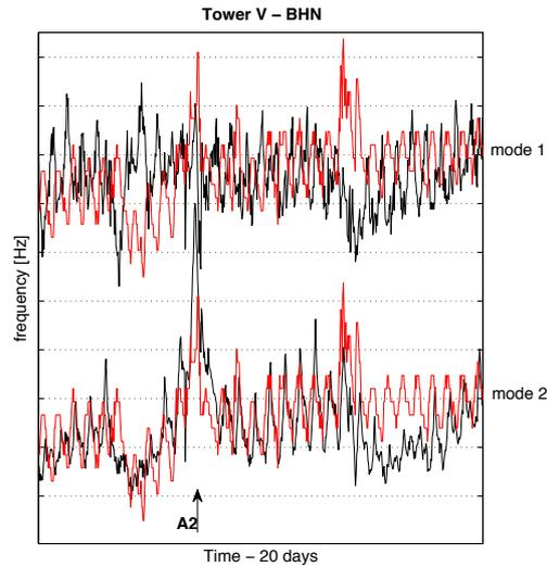
**Figure 5.** Zoom (20 days) of the frequency variations (black lines) for the longitudinal direction of the V tower considering the first (upper row) and second (lower row) modes, compared to the external temperature (red line) recorded at 10 km far away, at the Beirut airport. Value (Y-axis) are in Hz.
