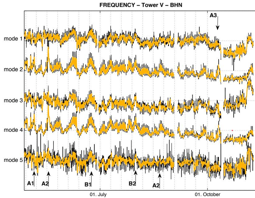
**Figure 3.** Frequency variations of the five first modes considering the longitudinal direction of the V tower. Yellow lines correspond to the smoothed variation, computed as the mean value of the frequency within a sliding windows (5 hours length). Value (Y-axis) are in Hz.
