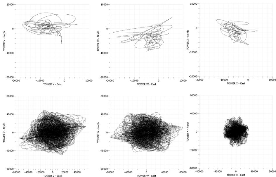
**Figure 6.** Ambient noise recording in the three towers. Upper row: filtered below 0.05 Hz. Lower row: Filtered around the fundamental frequency (0.6-1 Hz). Amplitude are in counts.
