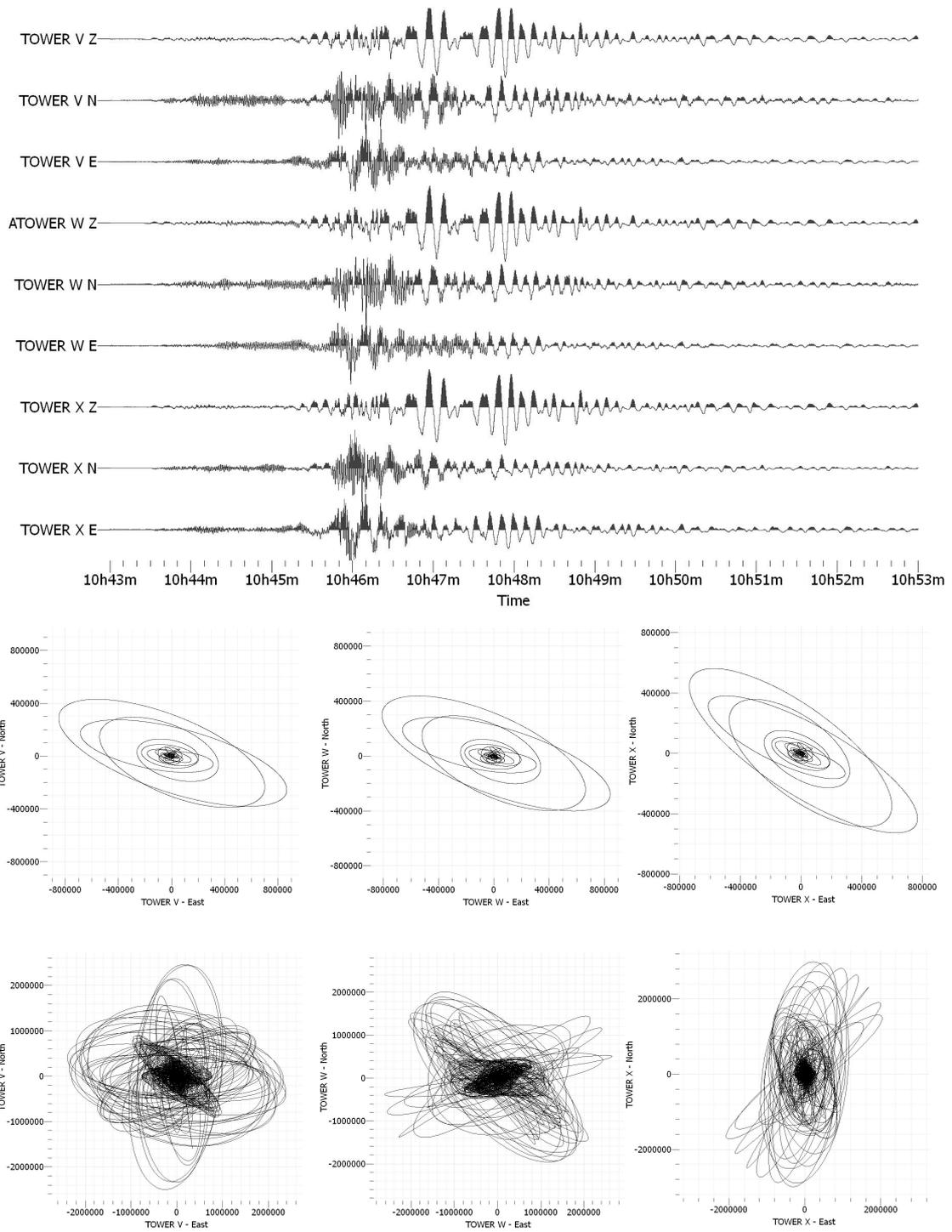
**Figure 7.** The records of the Van earthquake in the towers. Upper row: the 9 traces of the Van earthquake recorded in the towers. Middle row: the motion filtered below 0.05Hz. The three towers behave as an ensemble. Lower row: the motion filtered around the fundamental frequency of each building. The amplitude remains of the same order, but the motion look more independent from each other. Amplitude are in counts.
