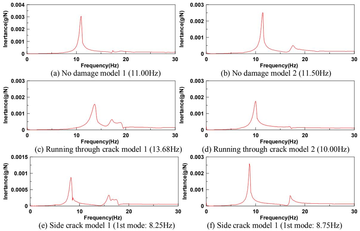
**Figure 6.** The results of impact hammer test
