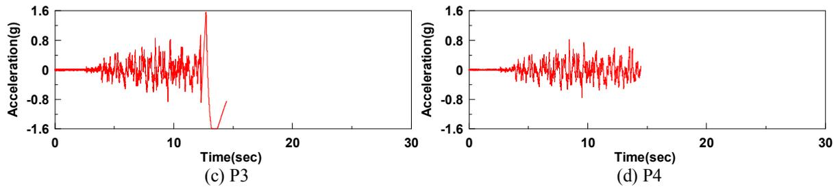
**Figure 8.** The acceleration time history response of running through crack model
