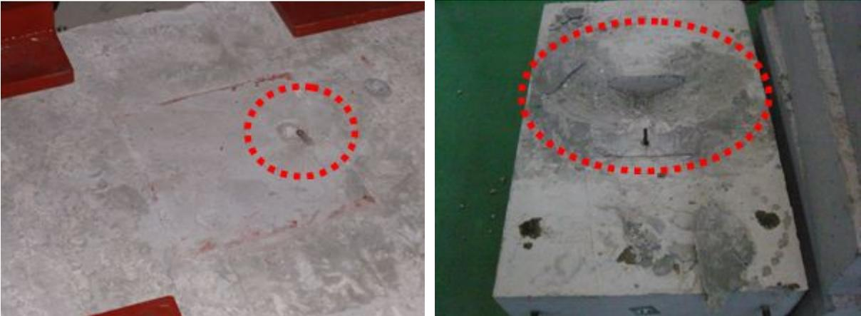
**Figure 5.** The failure shape of anchor bolt tensional and concrete breakout
