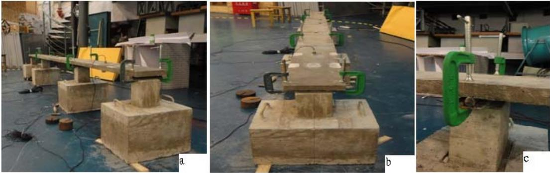
Figure 1. Three span reinforced concrete continuous beam model
