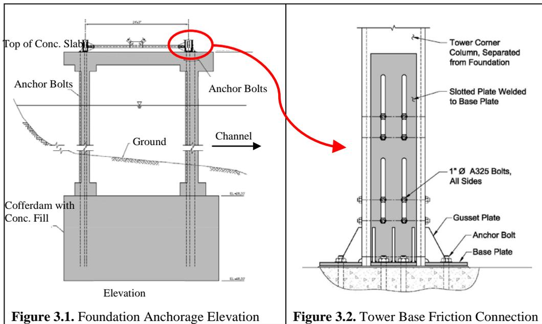
**Figure 3.1.** Foundation Anchorage Elevation
