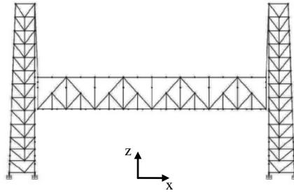
**Figure 2.1.** Schematic Elevation View of Fruitvale Ave Bridge, at Mid-Level Position
