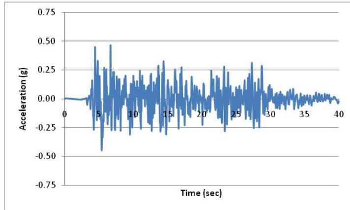
**Figure 3.4.** Horizontal Time History for Y-Direction Load Case
