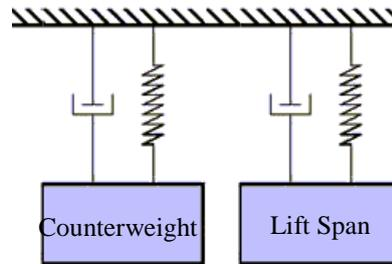
**Figure 2.7.** Schematic of Counterweight System Model
