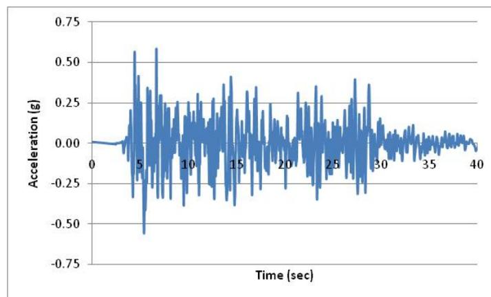
**Figure 3.5.** Horizontal Time History for X-Direction Load Case
