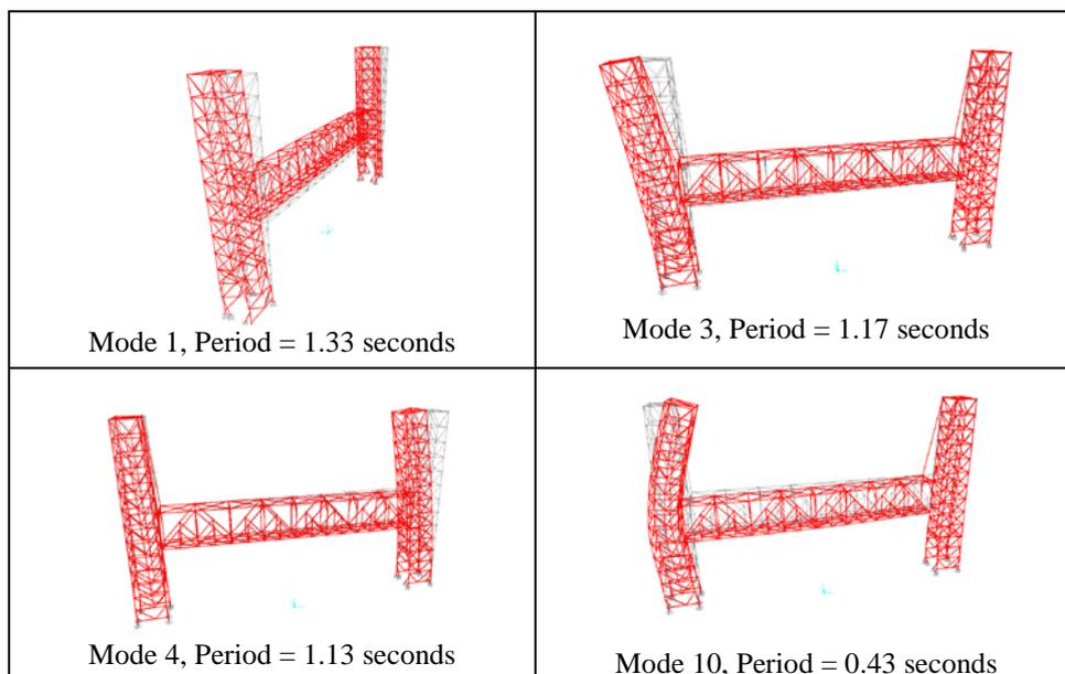
**Figure 2.5.** Selected Modes Shapes, Lift Span at Mid Position
