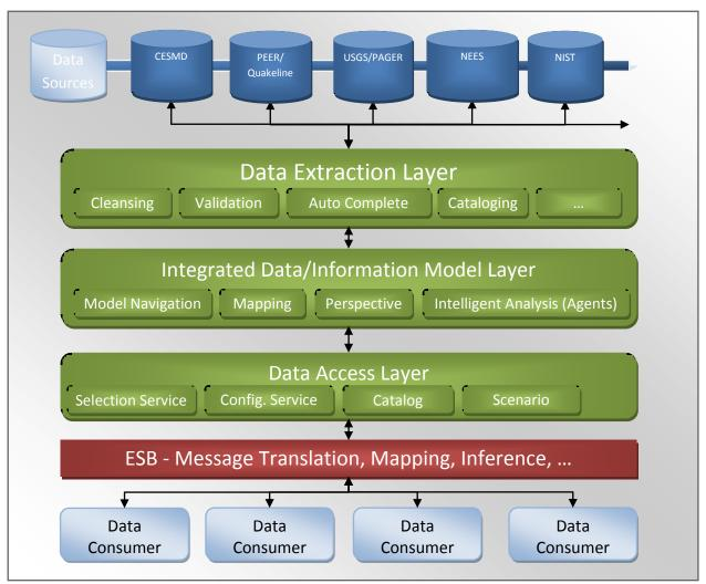
Figure 1. System Architecture for the Integrated Earthquake Data Environment
