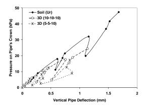
Figure 5. Soil pressure for improved geocell-reinforced and unreinforced installation
