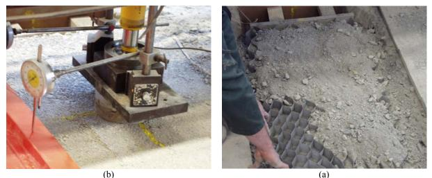
**Figure 3.** Test installations (a) Geocell installation beneath the footing, and (b) Loading plated located in centreline of the trench
