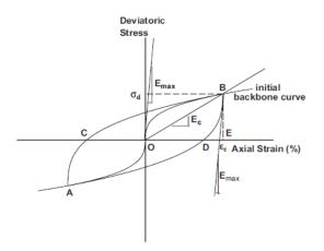
Figure 6. Schematic illustration of a symmetric stress-strain loop during the first cycle
