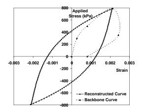
Figure 7. Reconstructed stress- strain loops for 3D (10-10-10)
