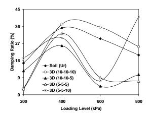
Figure 8. Damping ratios for all the tests at different loading levels.
