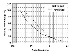
Figure 1. Grain size distribution curves for both native and backfill soils
