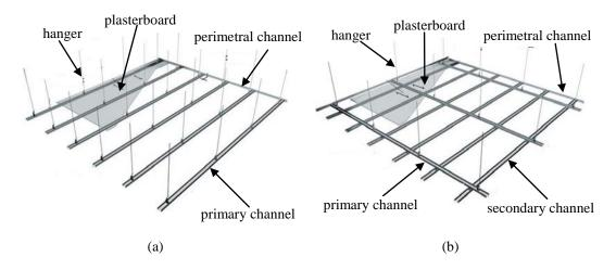
**Figure 2.1.** Suspended plasterboard continuous ceilings: (a) single frame ceiling (SFC); (b) double frame ceiling (DFC)
