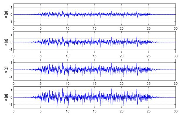
**Figure 2.4.** Input acceleration time histories for Y direction corresponding to SDS equal to 0.30g, 0.60g, 0.90g, 1.20g and 1.50g.
