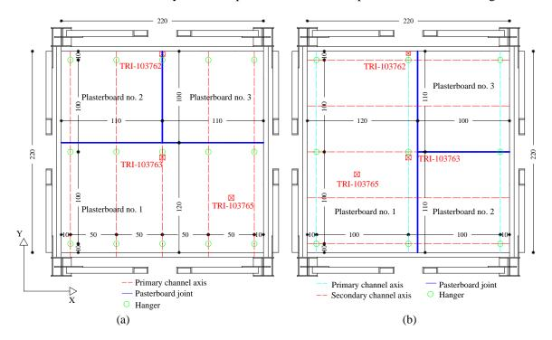
**Figure 2.3.** Triaxial accelerometers, plasterboard and hanger position in the case of single frame ceiling (a) and double frame ceiling (b) specimen
