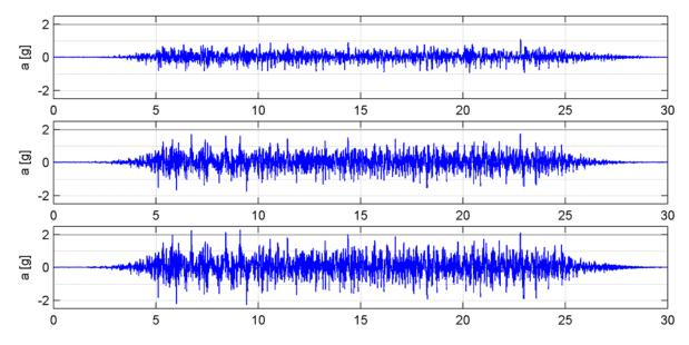
**Figure 3.1.** Acceleration time histories recorded on the ceiling (Accelerogram no. 103763) for single frame ceiling (SFC) for the intensity levels corresponding to SDS equal to 0.30g, 0.60g, 0.90g, 1.20g and 1.50g.
