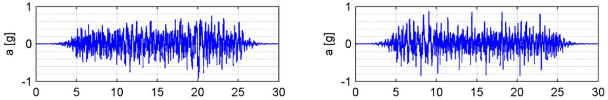
**Figure 2.5.** Input acceleration time histories for partition in-plane direction (X dir) and out-of-plane direction (Y dir) corresponding to SDS equal to 0.10g, 0.15g, 0.22g, 0.30g, 0.45g, 0.60g, 0.90g and 1.05g.
