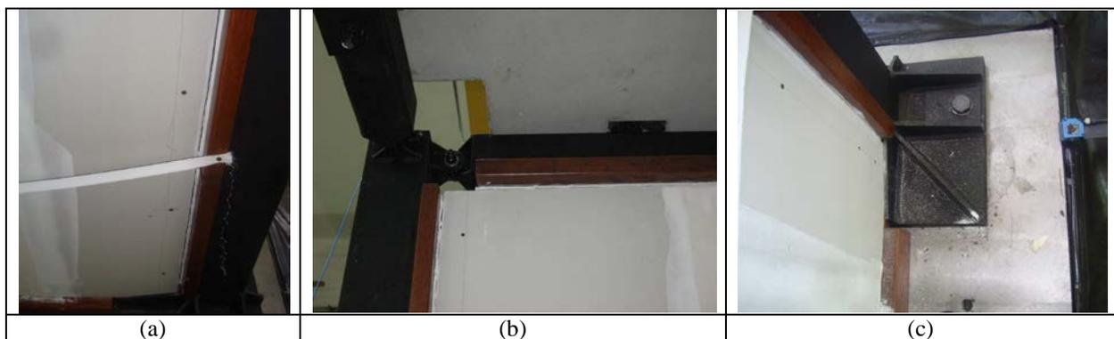
**Figure 4.1.** Photos of the light damages recorded after the bidirectional shake table tests: (a) and (b) acrylic silicon detachment, (c) chalk dust fall
