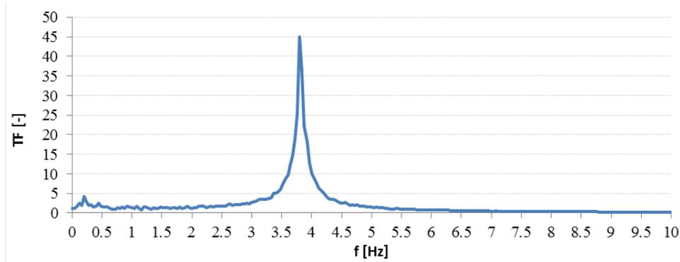
**Figure 3.2.** Transfer function generated by a white noise input on the bare structure.
