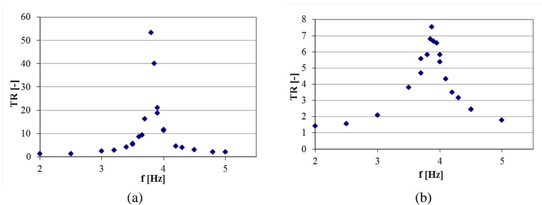
**Figure 3.1.** Transmissibility ratios curve of the bare steel frame (a) and for the infilled structure (b).
