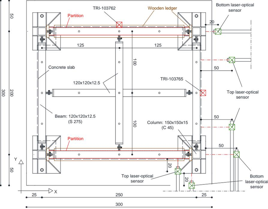
Figure 2.3. Location of the instrumentation: plan view
