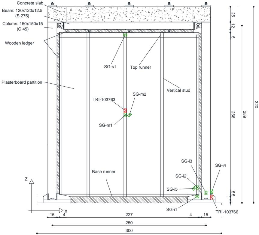
Figure 2.4. Location of the instrumentation: lateral view
