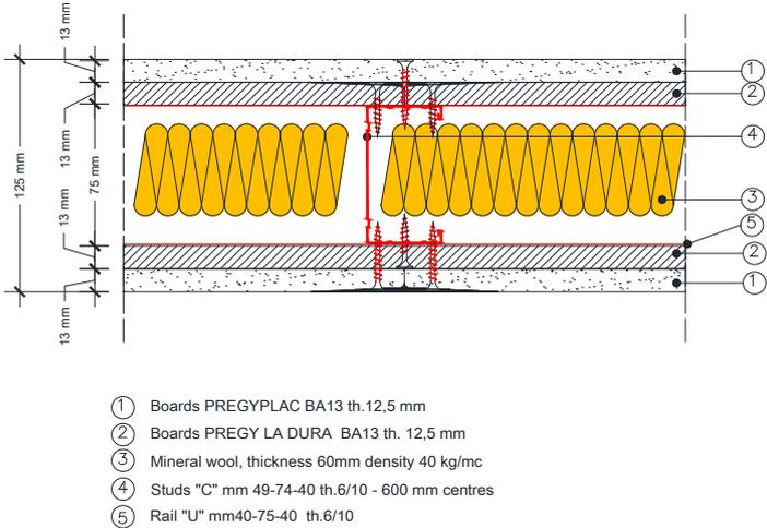
**Figure 2.2.** Cross section of the double layer of drywall partition
